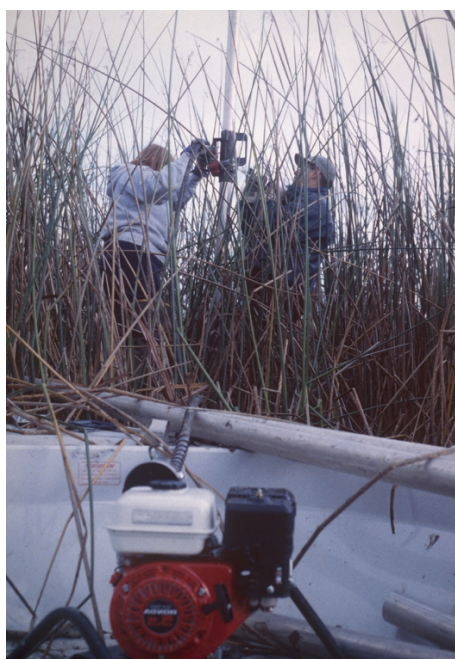
FIGURE 25. Insertion of base pipe using a vibracore system.
