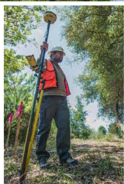
Right: DWR Engineer Sammy Naventhan of the South Central Region Office uses GPS rover to conduct field surveys at San Joaquin Parkway Trail project.
