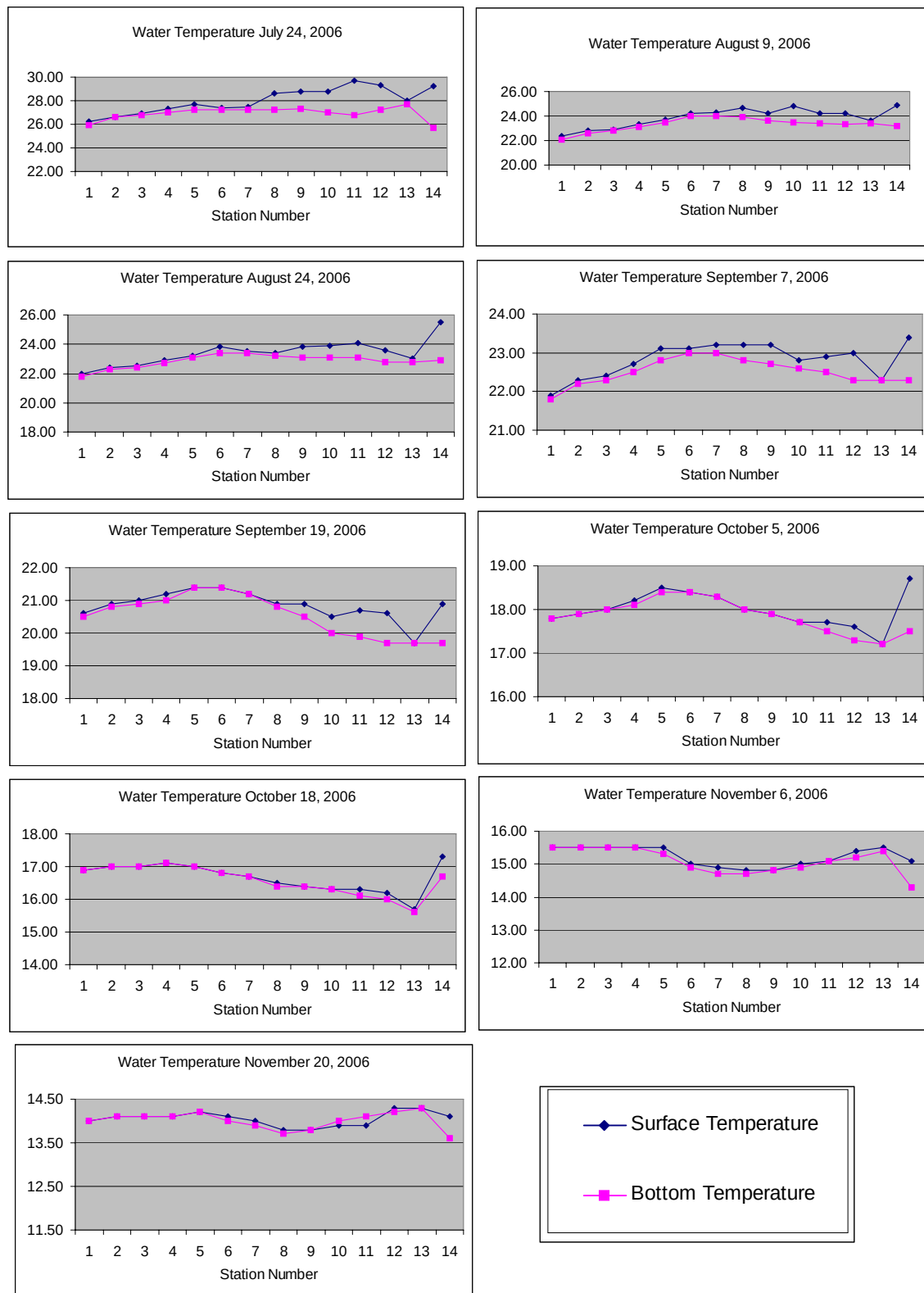
Figure 7-3 Water temperatures (°C) at 14 stations in the Stockton Ship Channel, summer/fall 2006
