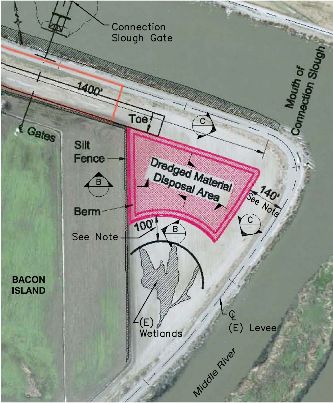
A DISPOSAL SITE PLAN NTS NOTE: SEE DWG G4 FOR LOCATION.
