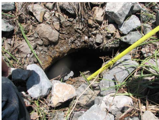
Tension crack at levee crest, Staten Island, Delta (Jul. 2007)
