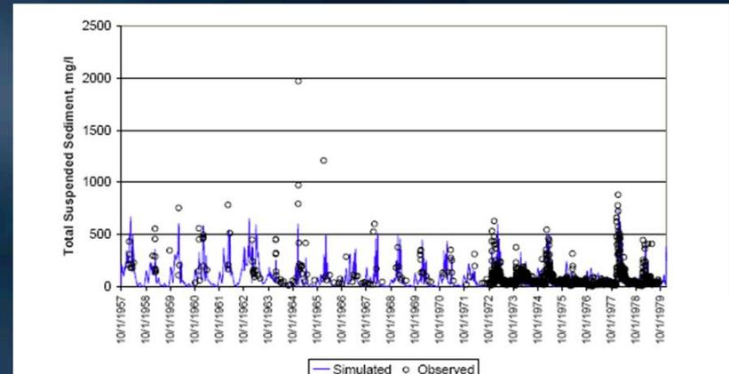
Figure 2-28 Simulated and observed total suspended sediment at Sacramento River at I Street Bridge
