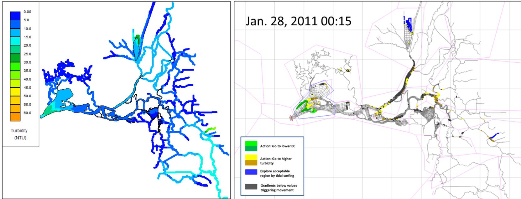
**Figure 12-162 Turbidity contours and particle location in the RMA model grid on Jan. 28, 2011.**
