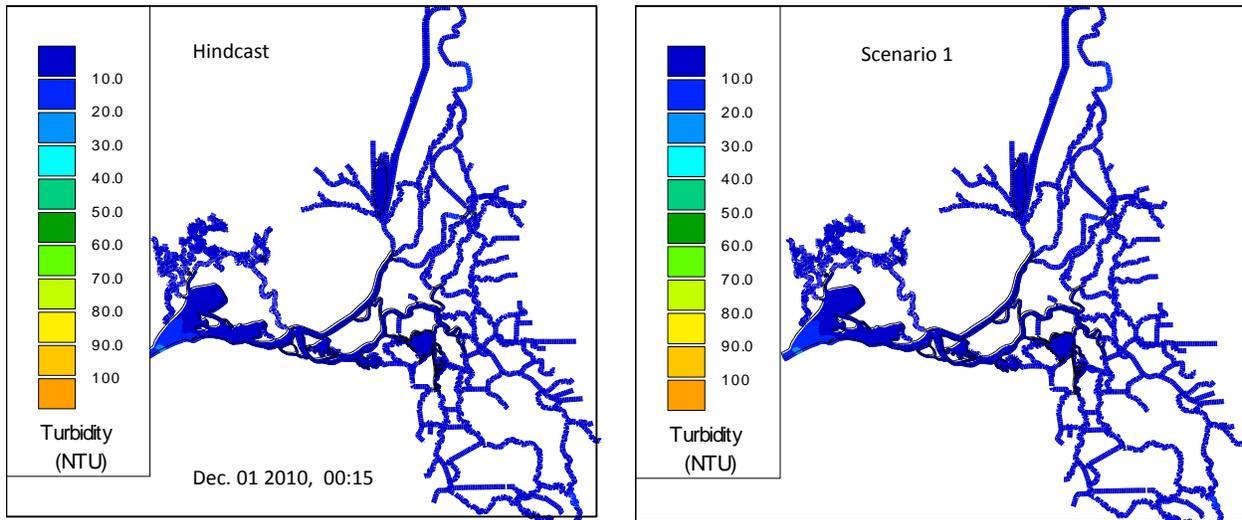
Figure 12-183 Comparison of turbidity contour results for the Hindcast (left) and the Modified Deriso scenario (right) on Dec. 01, 2010.
