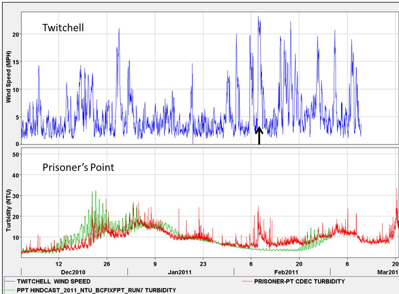
**Figure 12-180 Wind events, seen by wind velocity measured at the CIMIS/Twitchell station, in February increased turbidity at Prisoner's Point that wasn't captured in the modeling.**
