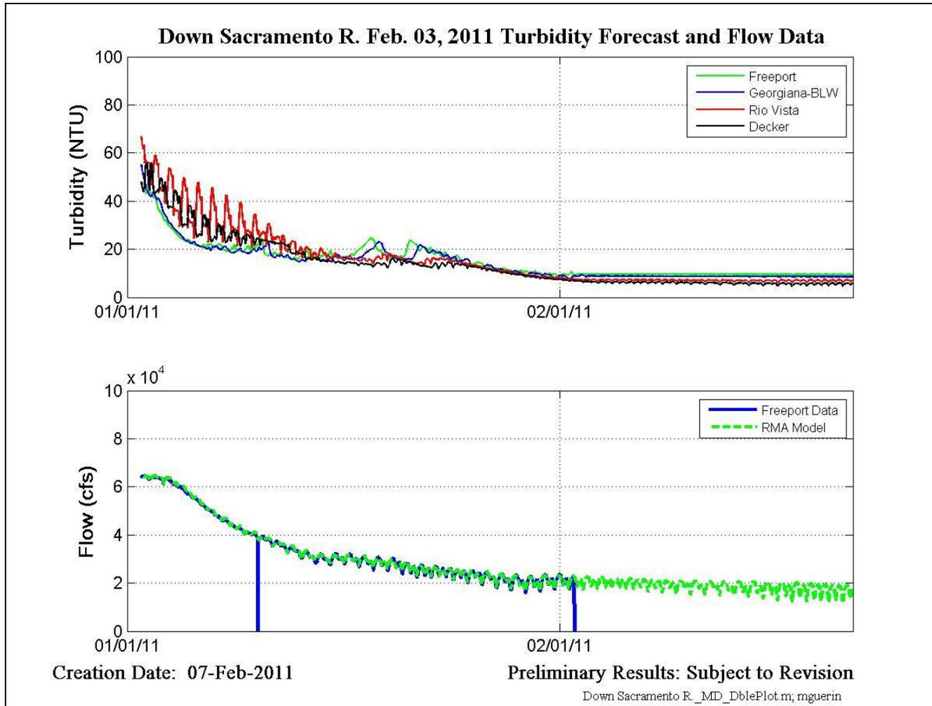
**Figure 12-150** Freeport turbidity boundary condition progression down the Sacramento R. (upper) along with the flow data and RMA model boundary conditions (lower) used during the modeled period. Forecast began on February 1<sup>st</sup>. End of flow data signals the beginning of the forecast.
