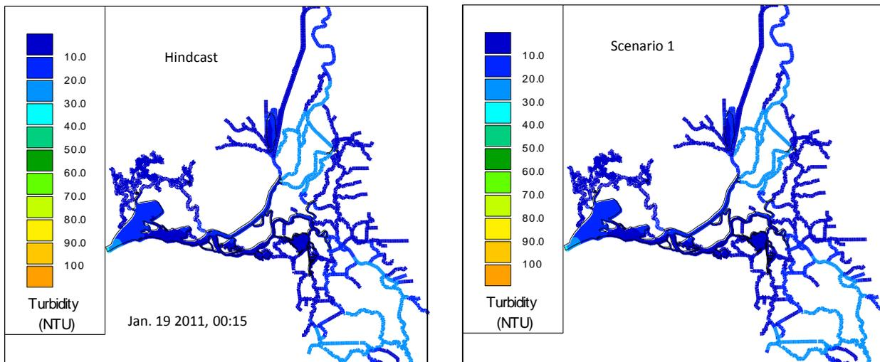
**Figure 12-197 Comparison of turbidity contour results for the Hindcast (left) and the Modified Deriso scenario (right) on Jan. 19, 2011.**
