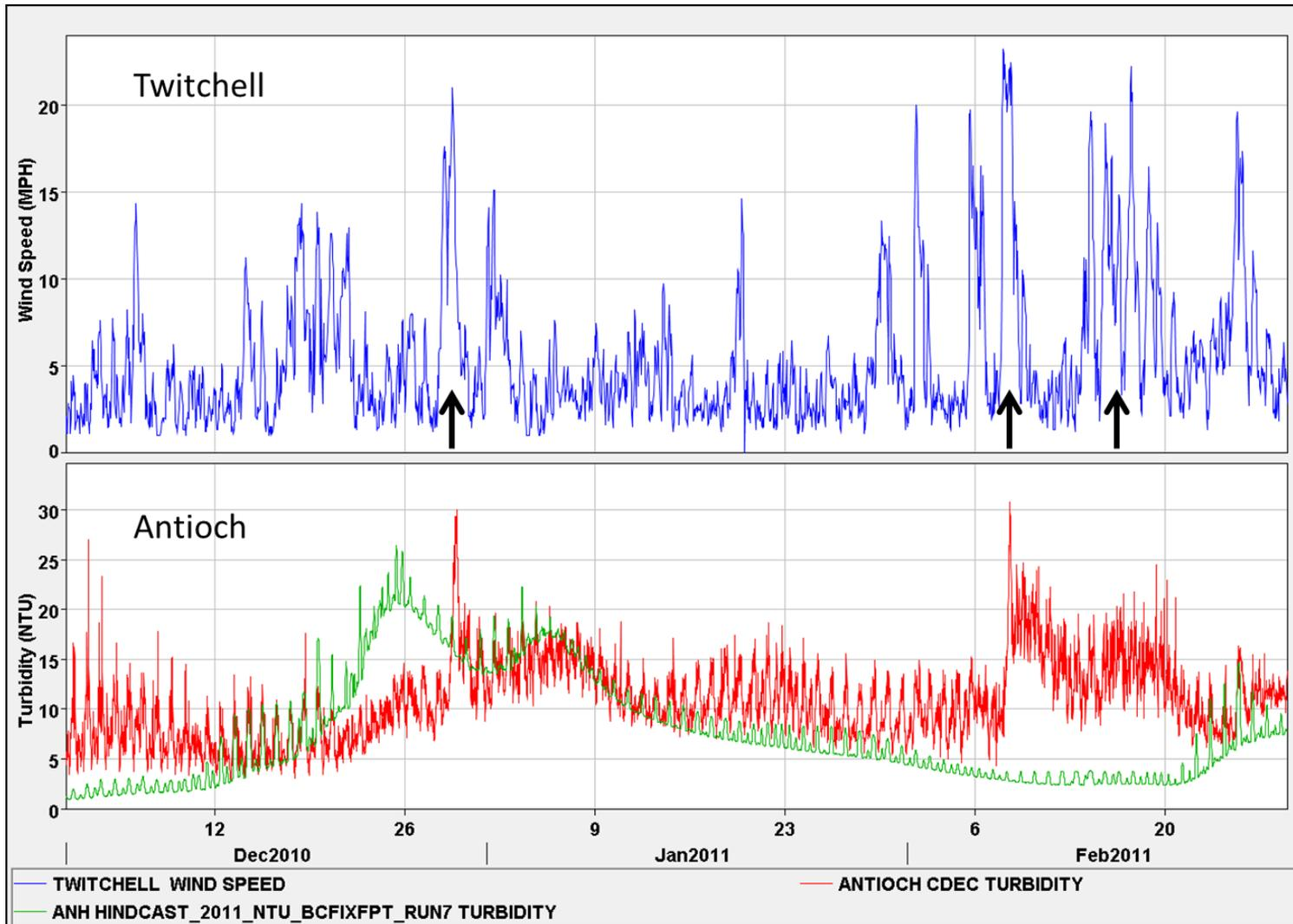
Figure 12-182 Wind events, recorded as increased wind velocity, measured at the CIMIS/Twitchell station in February increased turbidity at Antioch that wasn't captured in the modeling.
