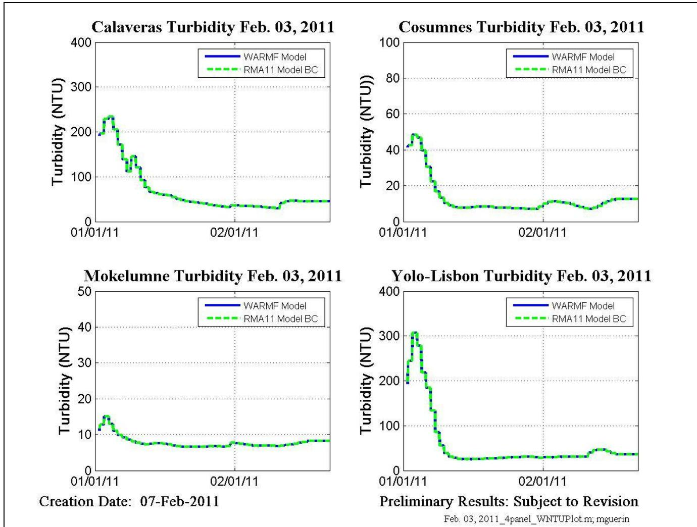
Figure 12-147 Turbidity boundary conditions used in the model along with the WARMF model output. Note difference in vertical scales.
