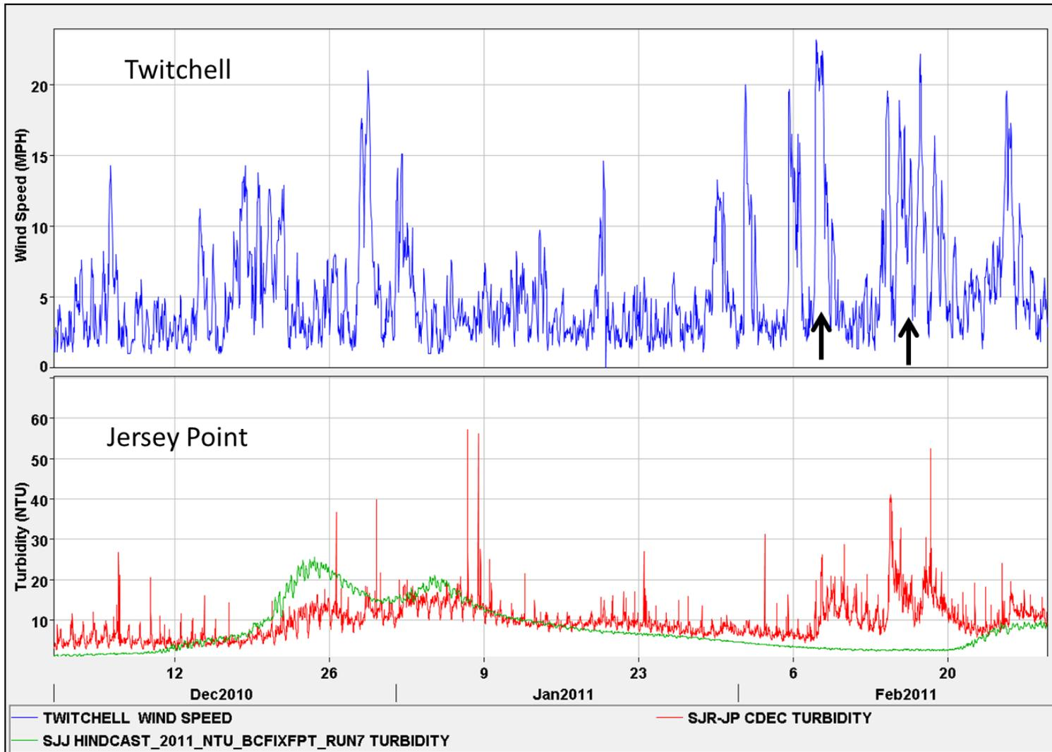
Figure 12-181 Wind events, seen by wind velocity measured at the CIMIS/Twitchell station, in February increased turbidity at Jersey Point that wasn't captured in the modeling.
