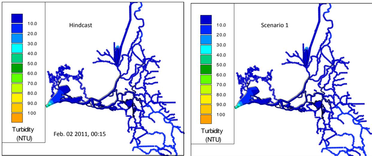
**Figure 12-201 Comparison of turbidity contour results for the Hindcast (left) and the Modified Deriso scenario (right) on Feb. 02, 2011.**
