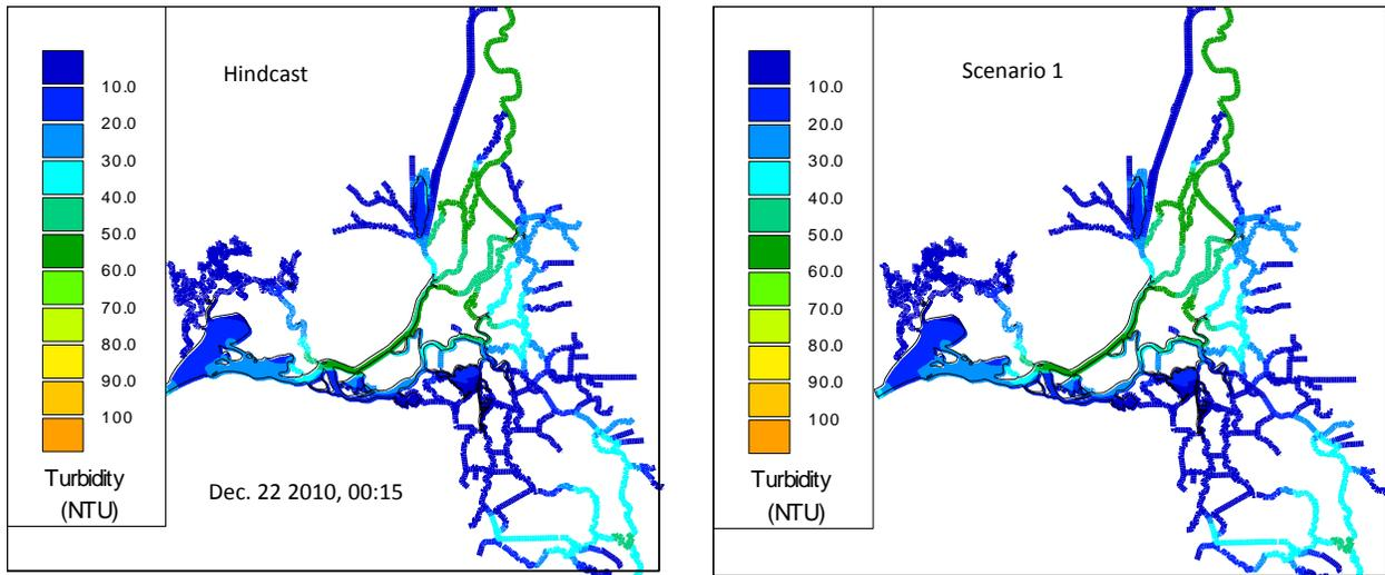
**Figure 12-189 Comparison of turbidity contour results for the Hindcast (left) and the Modified Deriso scenario (right) on Dec. 22, 2010.**
