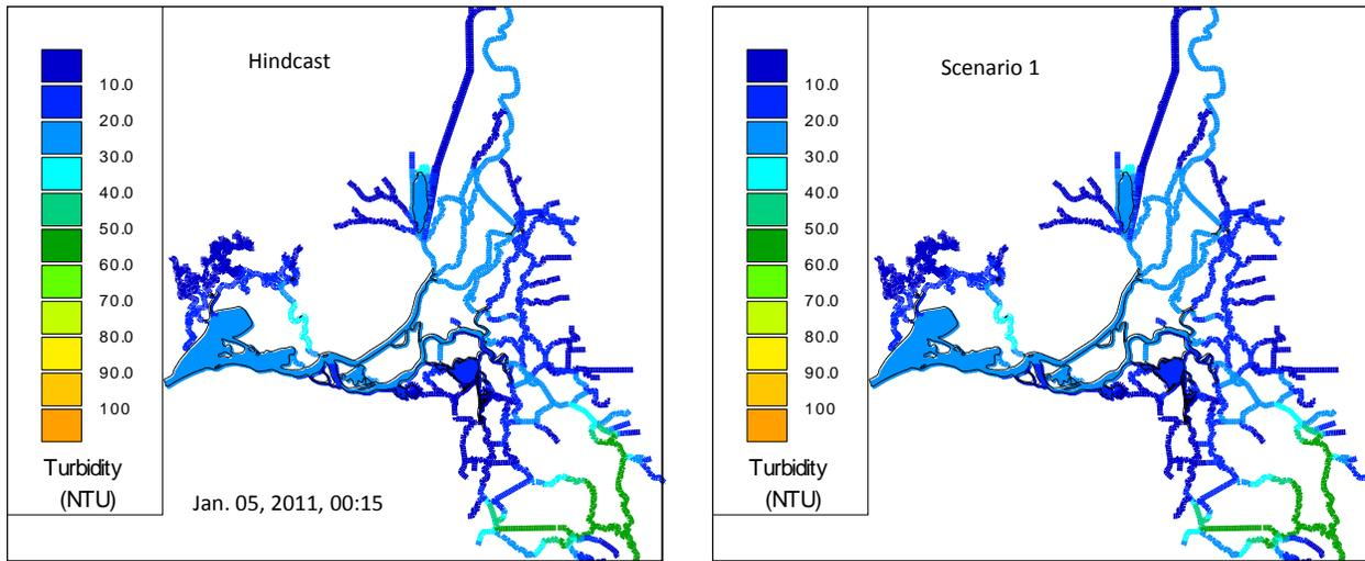
**Figure 12-193 Comparison of turbidity contour results for the Hindcast (left) and the Modified Deriso scenario (right) on Jan. 05, 2011.**
