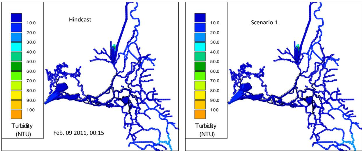
**Figure 12-203 Comparison of turbidity contour results for the Hindcast (left) and the Modified Deriso scenario (right) on Feb. 09, 2011.**
