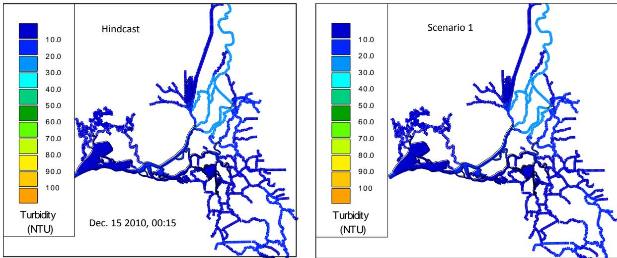
**Figure 12-187 Comparison of turbidity contour results for the Hindcast (left) and the Modified Deriso scenario (right) on Dec. 15, 2010.**
