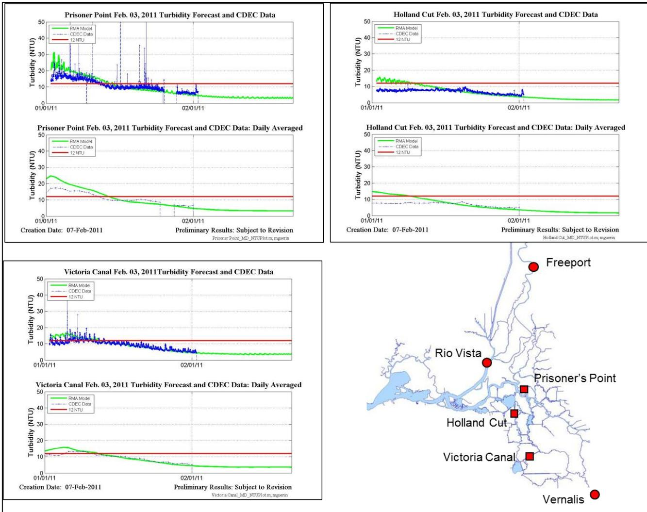
Figure 12-148 Modeled turbidity and data at the three compliance locations. Both 15-min model output and data and daily averaged plots are shown. Red line illustrates the 12-NTU compliance value.
