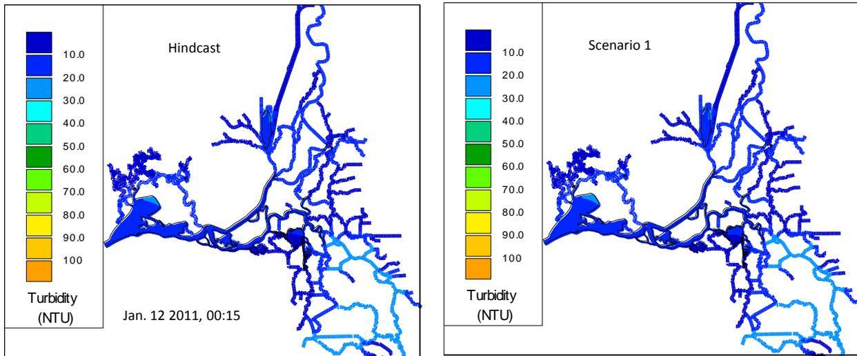
**Figure 12-195 Comparison of turbidity contour results for the Hindcast (left) and the Modified Deriso scenario (right) on Jan. 12, 2011.**
