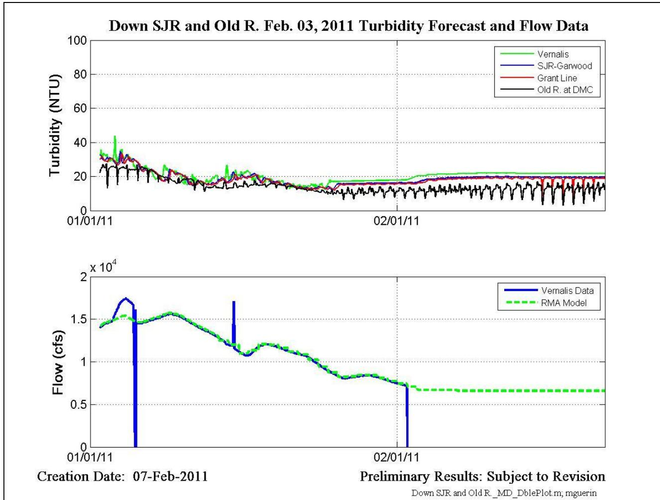
**Figure 12-151 Progression of the turbidity boundary condition from Vernalis down the San Joaquin R. to Garwood, and down Old River (upper plot). Flow data and RMA model boundary condition at Vernalis are shown in the lower plot. Forecast began on Jan 25<sup>th</sup>. End of flow data signals the beginning of the forecast.**
