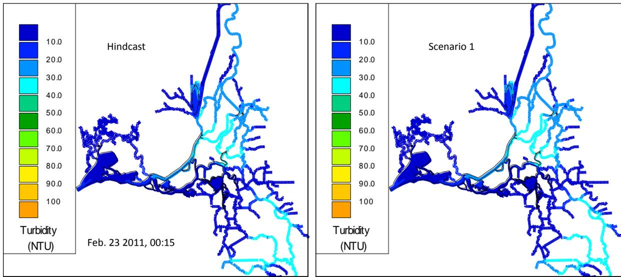
**Figure 12-207 Comparison of turbidity contour results for the Hindcast (left) and the Modified Deriso scenario (right) on Feb. 23, 2011.**
