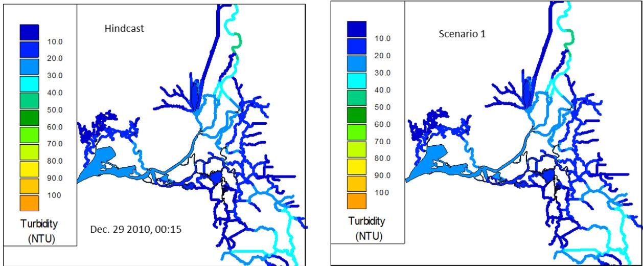
**Figure 12-191 Comparison of turbidity contour results for the Hindcast (left) and the Modified Deriso scenario (right) on Dec. 29, 2010.**
