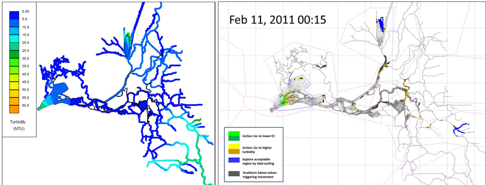
**Figure 12-164 Turbidity contours and particle location in the RMA model grid on Feb 11, 2011.**
