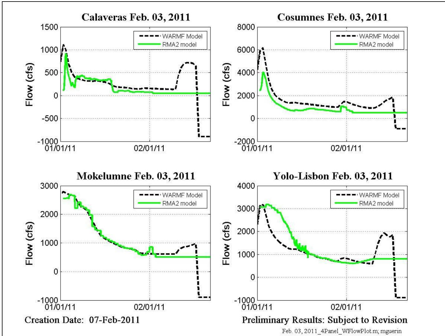
Figure 12-146 Four flow boundary conditions used in the model along with the WARMF model output.
