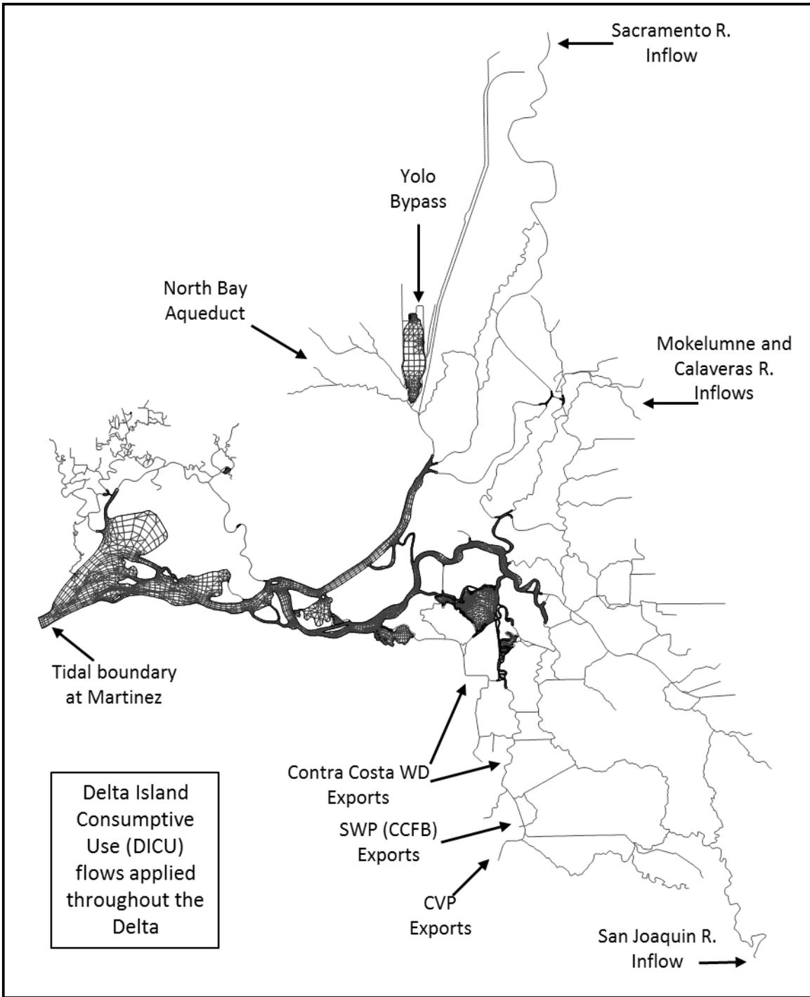
**Figure 3-3 Finite element model configuration of the Sacramento – San Joaquin Delta.**
