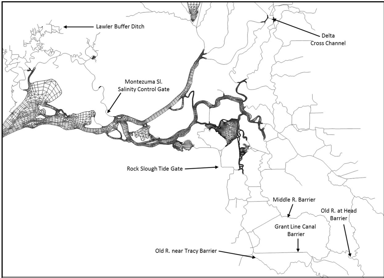
**Figure 3-4 Approximate gate and barrier locations in the RMA grid.**
