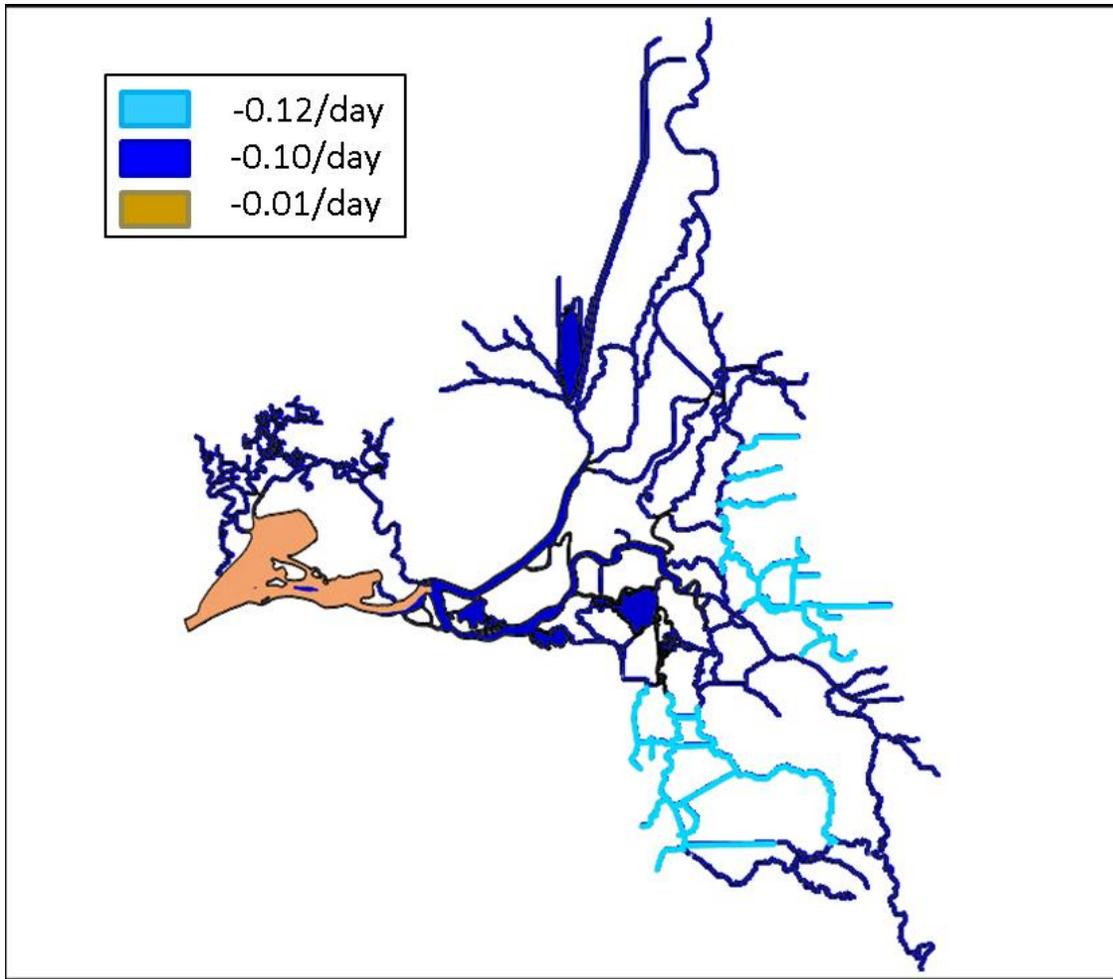
**Figure 3-5 Decay values and regions used in the WY2010 turbidity model. The previous turbidity model had a single decay value of -0.5/day.**
