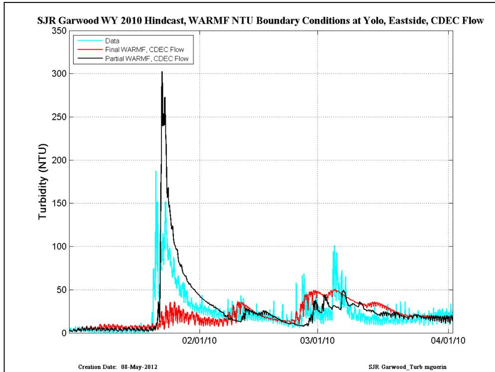
Figure 3 CDEC data (cyan) compared with RMA simulations run with Final WARMF (red) and Partial WARMF (black) – results are shown at Garwood on the San Joaquin River in WY2010.
