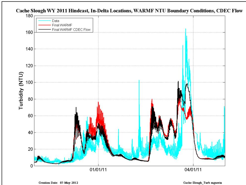
Figure 40 CDEC data (cyan) compared with RMA simulations run with Final WARMF (red) and Final WARMF and CDEC flows (black) – results are shown in Cache Slough at Ryer in WY2011.
