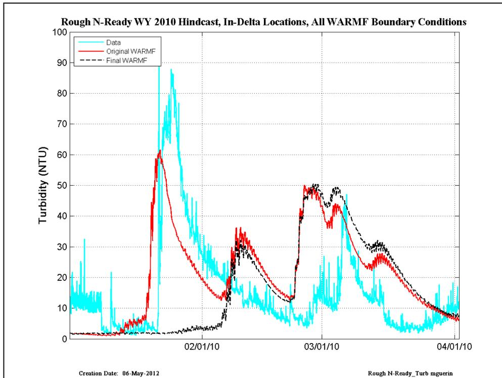
Figure 22 CDEC data (cyan) compared with RMA simulations run with original WARMF (red) and Final WARMF (black) – results are shown at Rough N’Ready Island on the San Joaquin River in WY2010.
