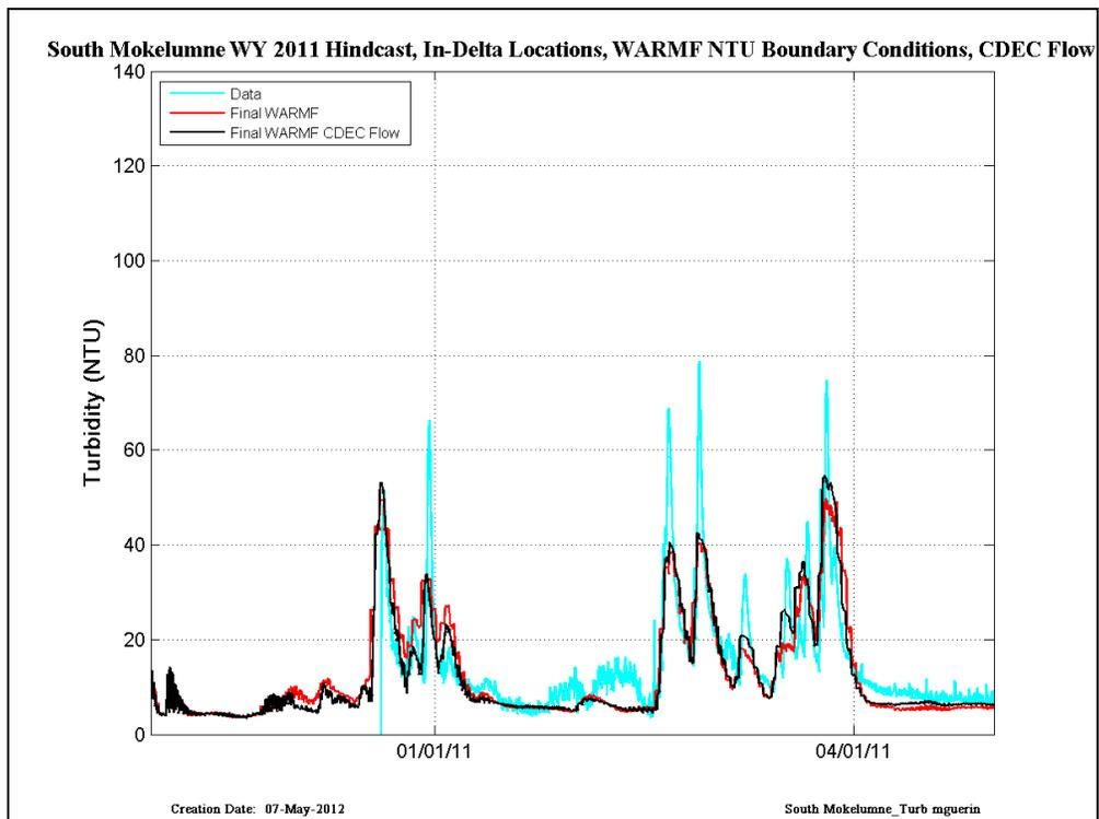
Figure 54 CDEC data (cyan) compared with RMA simulations run with Final WARMF (red) and Final WARMF and CDEC flows (black) – results are shown at the South Mokelumne in WY2011.
