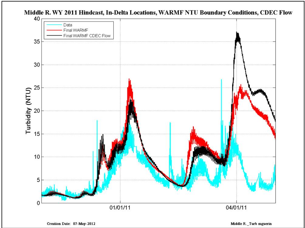
Figure 50 CDEC data (cyan) compared with RMA simulations run with Final WARMF (red) and Final WARMF and CDEC flows (black) – results are shown in Middle River in WY2011.
