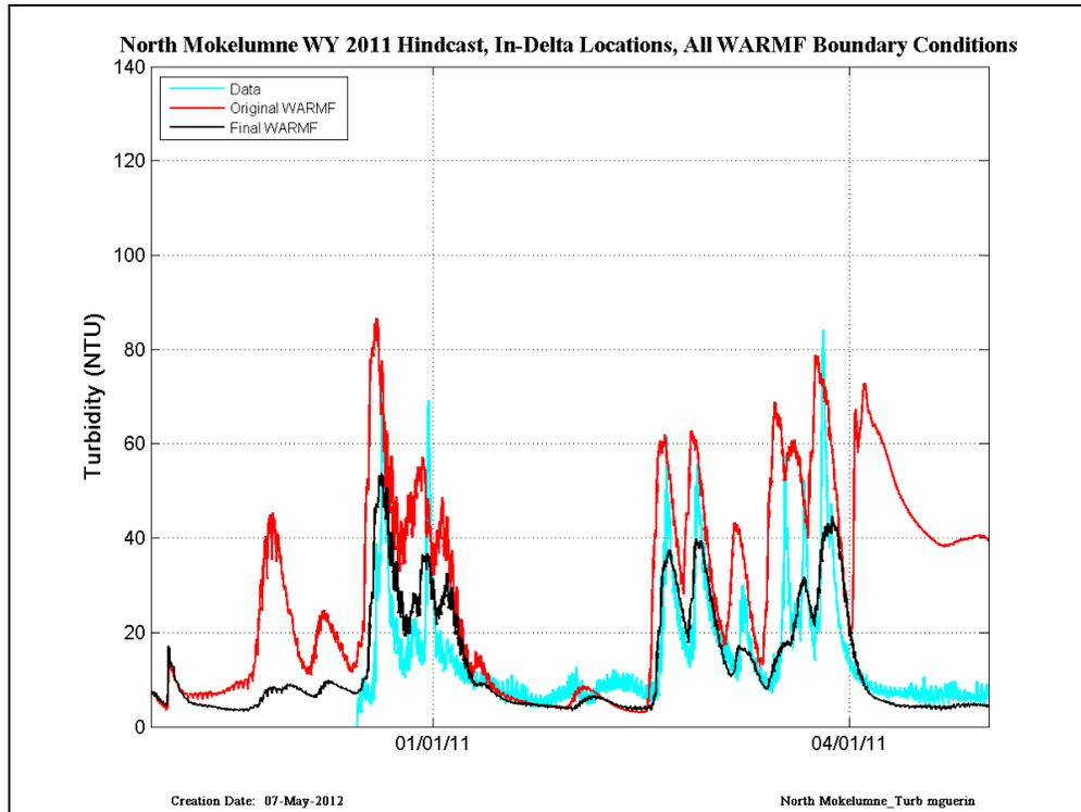
Figure 37 CDEC data (cyan) compared with RMA simulations run with original WARMF (red) and Final WARMF (black) – results are shown at the North Mokelumne location in WY2011.
