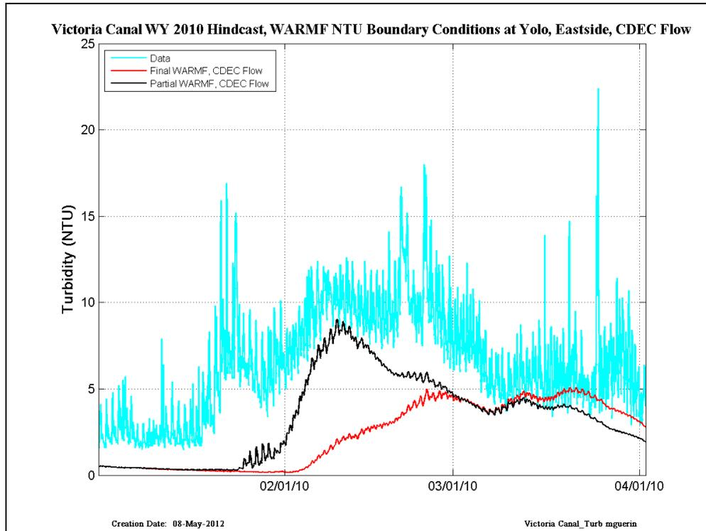
Figure 7 CDEC data (cyan) compared with RMA simulations run with Final WARMF (red) and Partial WARMF (black) – results are shown at Victoria Canal in WY2010.
