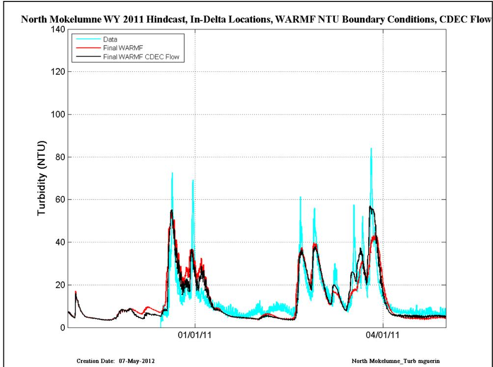
Figure 53 CDEC data (cyan) compared with RMA simulations run with Final WARMF (red) and Final WARMF and CDEC flows (black) – results are shown at the North Mokelumne in WY2011.
