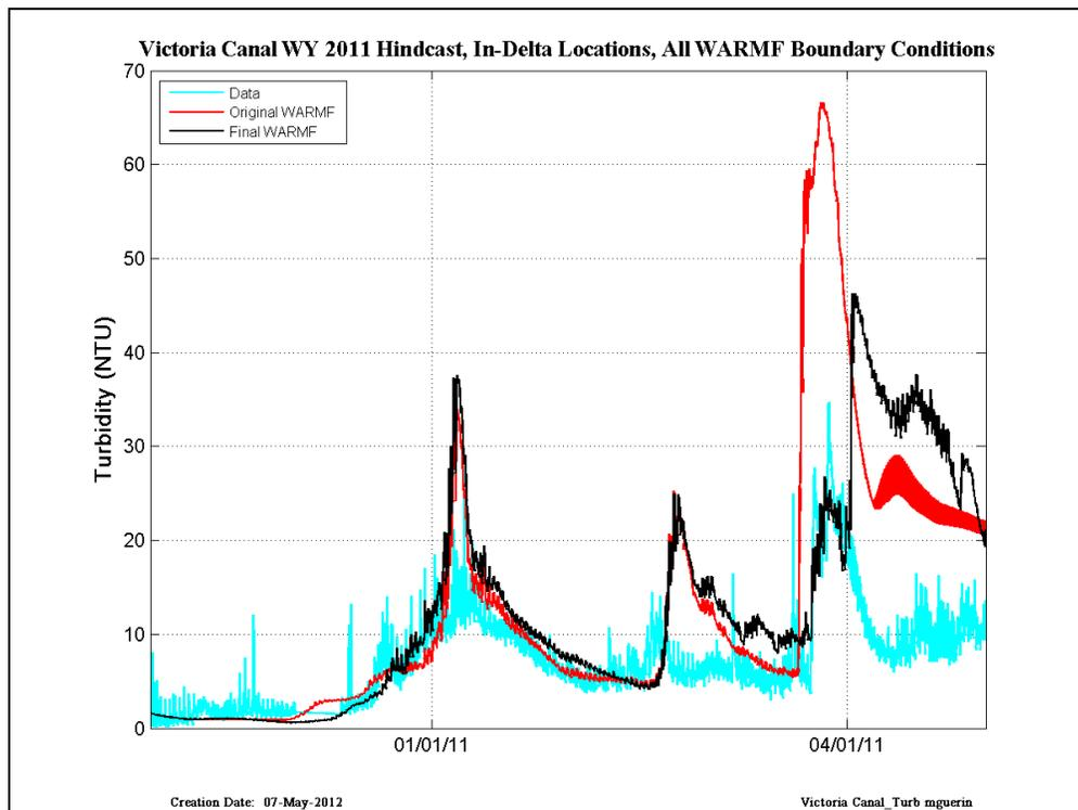
Figure 36 CDEC data (cyan) compared with RMA simulations run with original WARMF (red) and Final WARMF (black) – results are shown at Victoria Canal in WY2011.
