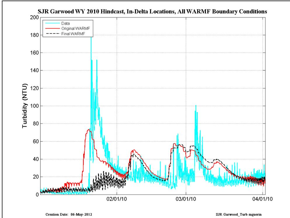
Figure 21 CDEC data (cyan) compared with RMA simulations run with original WARMF (red) and Final WARMF (black) – results are shown at Garwood on the San Joaquin River in WY2010.
