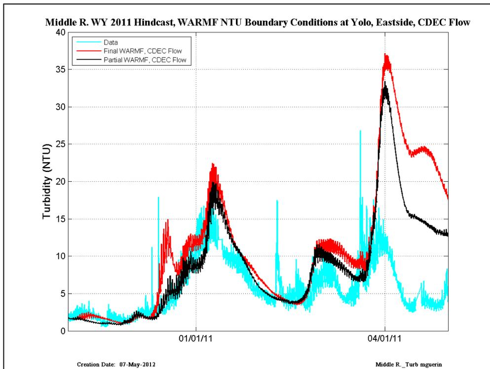
Figure 13 CDEC data (cyan) compared with RMA simulations run with Final WARMF (red) and Partial WARMF (black) – results are shown at the Middle River location in WY2011.
