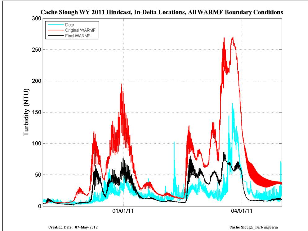
Figure 29 CDEC data (cyan) compared with RMA simulations run with original WARMF (red) and Final WARMF (black) – results are shown in Cache Slough at Ryer in WY2011.
