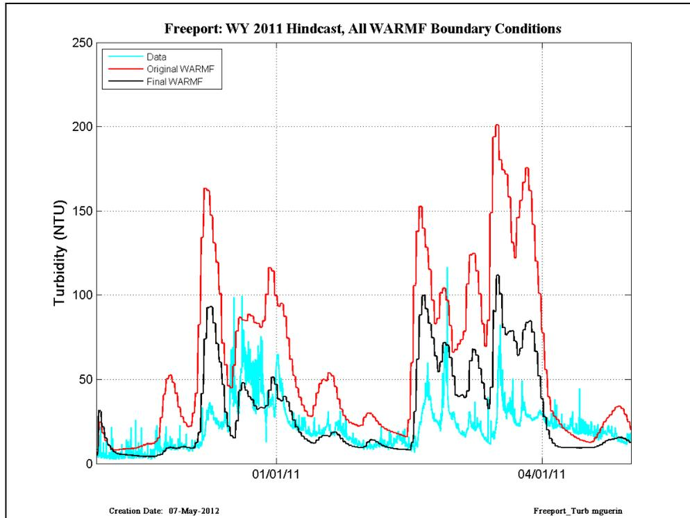
Figure 27 CDEC data (cyan) compared with RMA simulations run with original WARMF (red) and Final WARMF (black) – results are shown at Freeport in WY2011.
