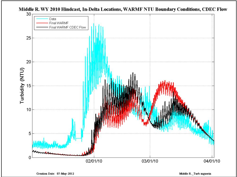
Figure 49 CDEC data (cyan) compared with RMA simulations run with Final WARMF (red) and Final WARMF and CDEC flows (black) – results are shown in Middle River in WY2010.
