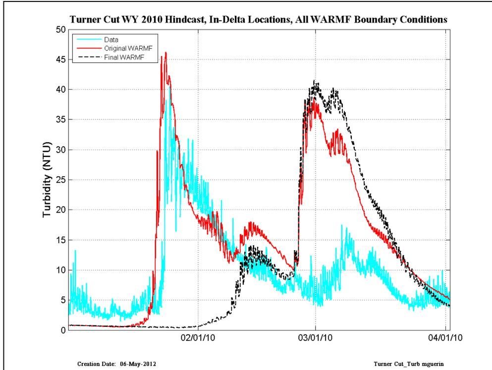
Figure 25 CDEC data (cyan) compared with RMA simulations run with original WARMF (red) and Final WARMF (black) – results are shown at Turner Cut in WY2010.
