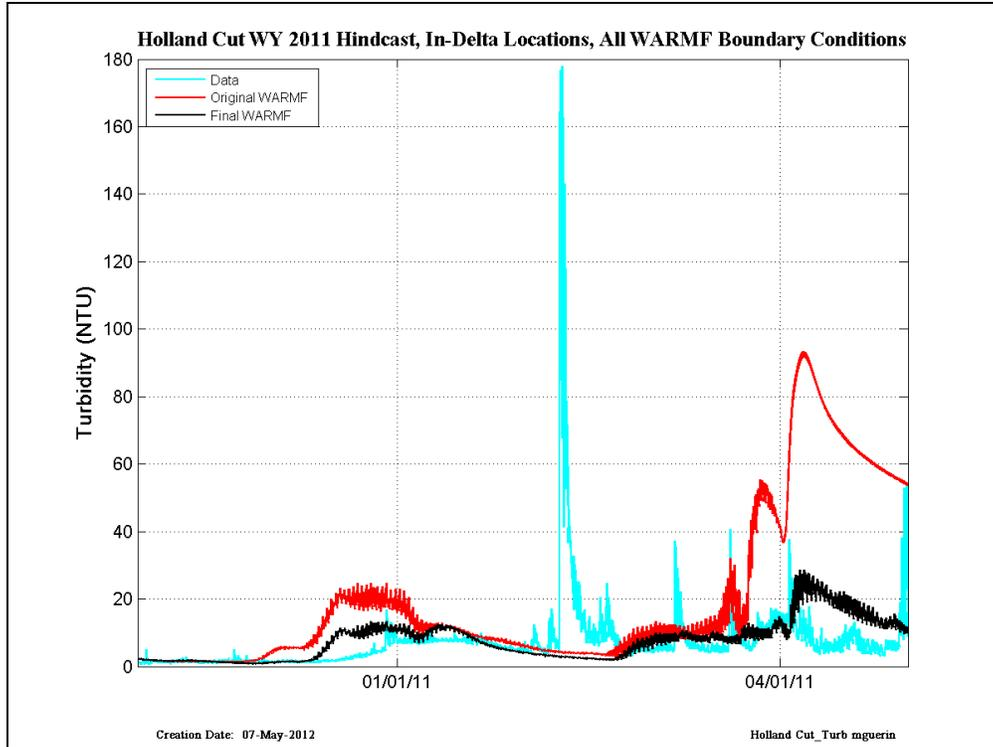
Figure 33 CDEC data (cyan) compared with RMA simulations run with original WARMF (red) and Final WARMF (black) – results are shown at Holland Cut in WY2011.
