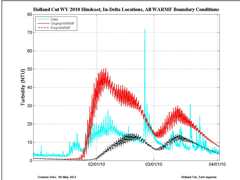
Figure 23 CDEC data (cyan) compared with RMA simulations run with original WARMF (red) and Final WARMF (black) – results are shown at Holland Cut in WY2010.
