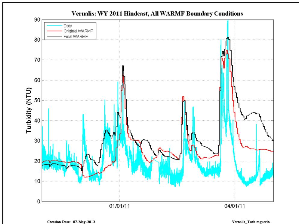
Figure 28 CDEC data (cyan) compared with RMA simulations run with original WARMF (red) and Final WARMF (black) – results are shown at Vernalis in WY2011.
