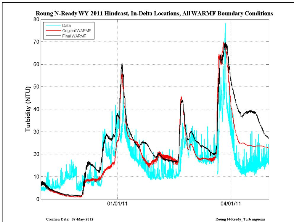
Figure 32 CDEC data (cyan) compared with RMA simulations run with original WARMF (red) and Final WARMF (black) – results are shown at Rough N'Ready in WY2011.
