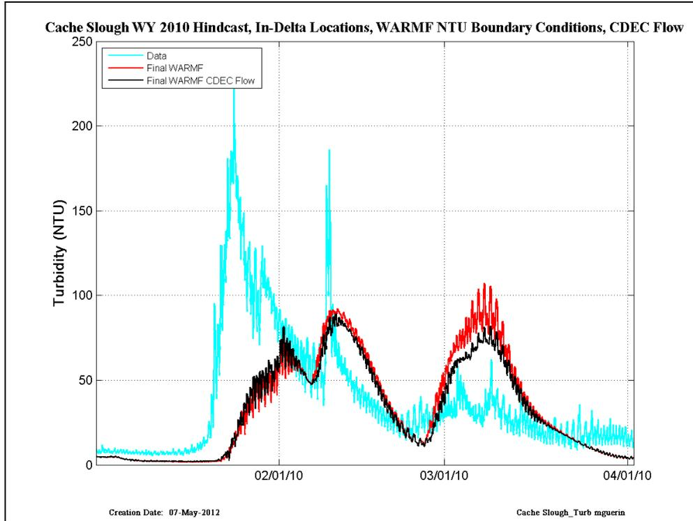
Figure 39 CDEC data (cyan) compared with RMA simulations run with Final WARMF (red) and Final WARMF and CDEC flows (black) – results are shown in Cache Slough at Ryer in WY2010.
