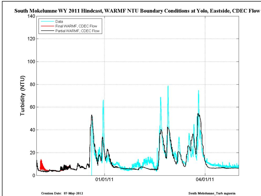
Figure 16 CDEC data (cyan) compared with RMA simulations run with Final WARMF (red) and Partial WARMF (black) – results are shown at the South Mokelumne River location in WY2011.
