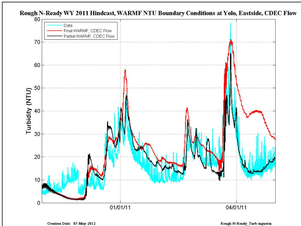
Figure 11 CDEC data (cyan) compared with RMA simulations run with Final WARMF (red) and Partial WARMF (black) – results are shown at Rough N'Ready Island on the san Joaquin River in WY2011.
