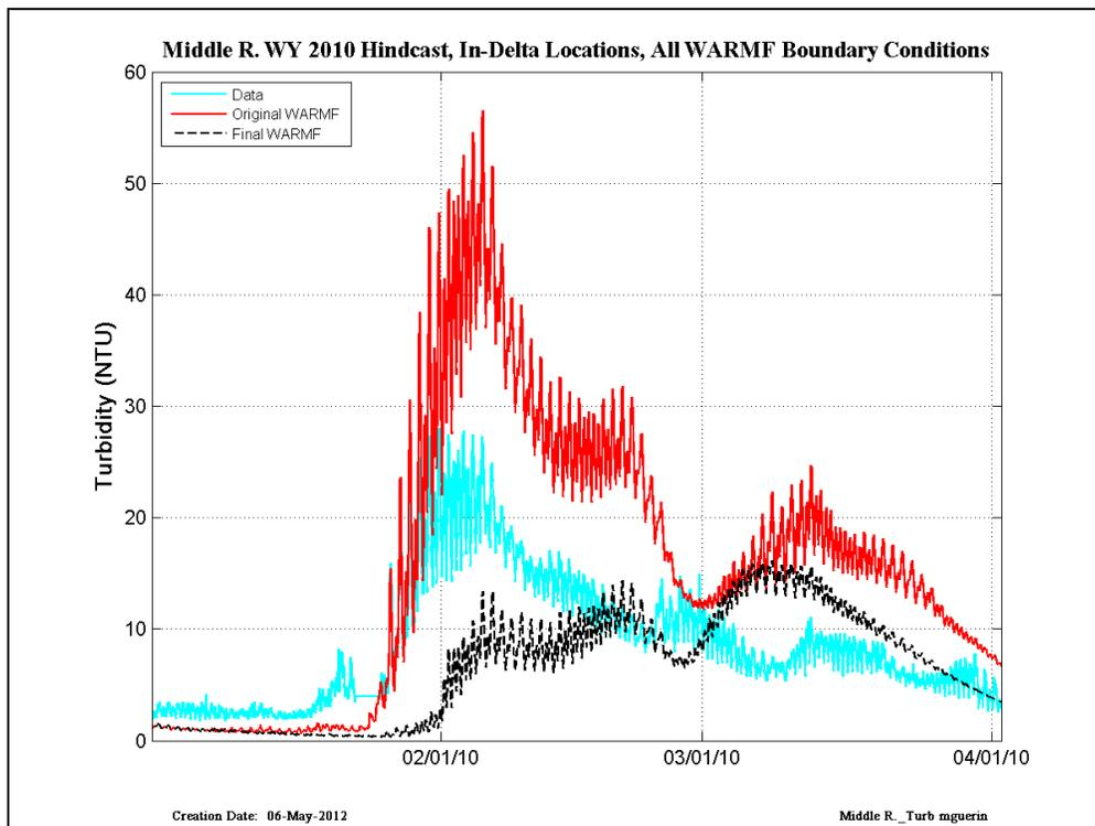
Figure 24 CDEC data (cyan) compared with RMA simulations run with original WARMF (red) and Final WARMF (black) – results are shown at the Middle River location in WY2010.
