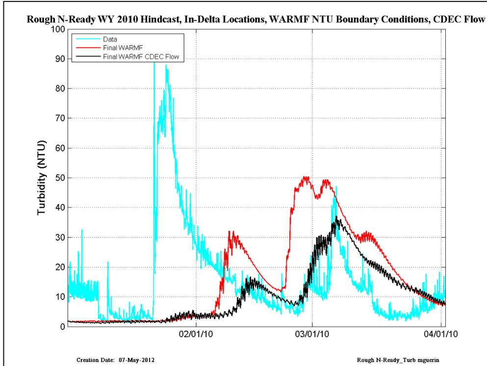
Figure 45 CDEC data (cyan) compared with RMA simulations run with Final WARMF (red) and Final WARMF and CDEC flows (black) – results are shown at Rough N’Ready on the San Joaquin River in WY2010.
