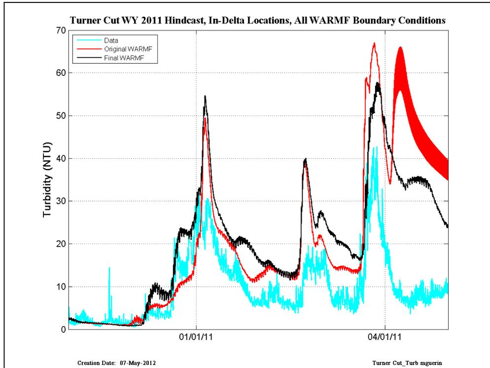
Figure 35 CDEC data (cyan) compared with RMA simulations run with original WARMF (red) and Final WARMF (black) – results are shown at Turner Cut in WY2011.
