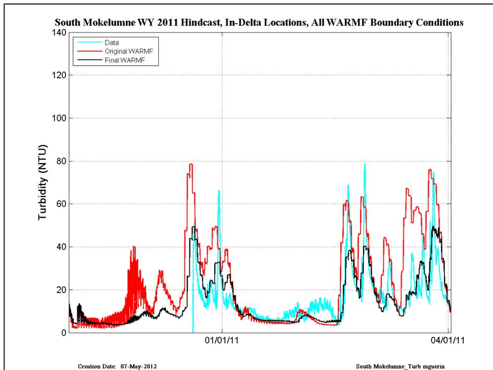
Figure 38 CDEC data (cyan) compared with RMA simulations run with original WARMF (red) and Final WARMF (black) – results are shown at the South Mokelumne location in WY2011.
