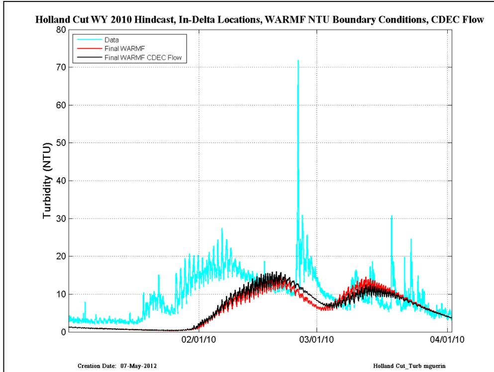
Figure 47 CDEC data (cyan) compared with RMA simulations run with Final WARMF (red) and Final WARMF and CDEC flows (black) – results are shown in Holland Cut in WY2010.
