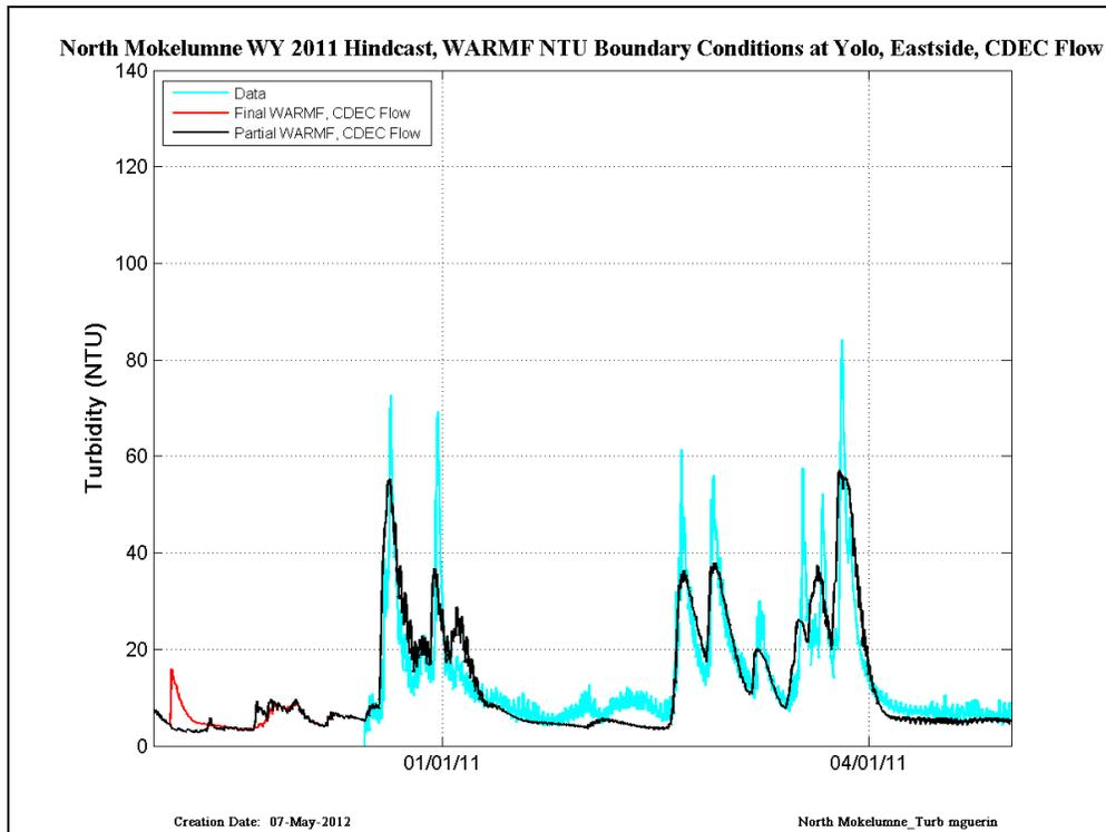
Figure 15 CDEC data (cyan) compared with RMA simulations run with Final WARMF (red) and Partial WARMF (black) – results are shown at the North Mokelumne River location in WY2011.
