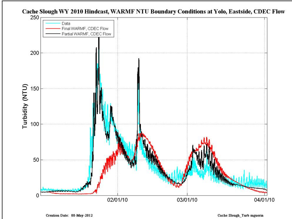
Figure 1 CDEC data (cyan) compared with RMA simulations run with Final WARMF (red) and Partial WARMF (black) – results are shown at Cache Slough at Ryer in WY2010.
