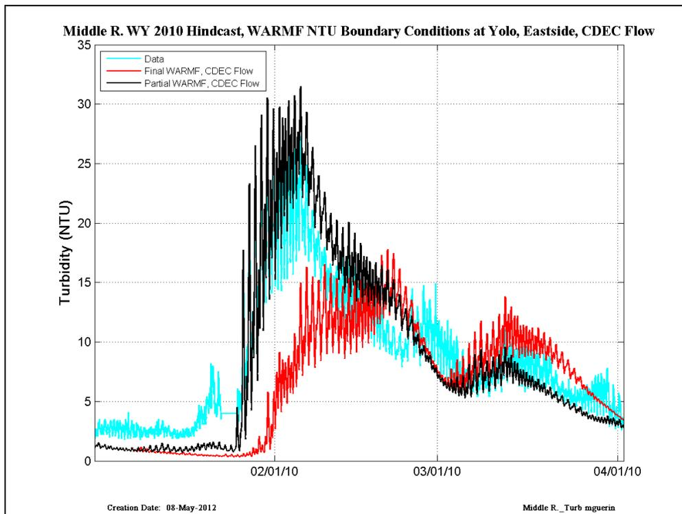
Figure 6 CDEC data (cyan) compared with RMA simulations run with Final WARMF (red) and Partial WARMF (black) – results are shown at the Middle River location in WY2010.
