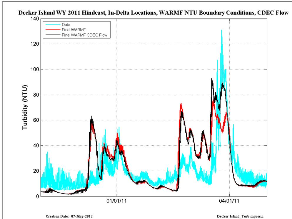
Figure 42 CDEC data (cyan) compared with RMA simulations run with Final WARMF (red) and Final WARMF and CDEC flows (black) – results are shown in Decker Island on the Sacramento River in WY2011.
