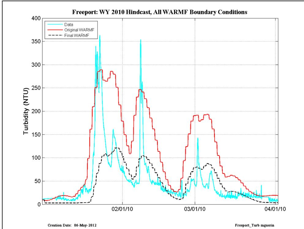
Figure 17 CDEC data (cyan) compared with RMA simulations run with original WARMF (red) and Final WARMF (black) – results are shown at Freeport in WY2010.
