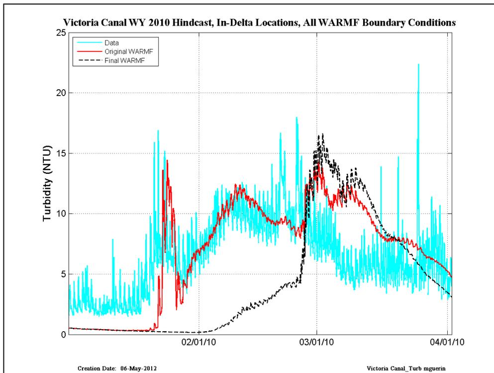
Figure 26 CDEC data (cyan) compared with RMA simulations run with original WARMF (red) and Final WARMF (black) – results are shown at Victoria Canal in WY2010.
