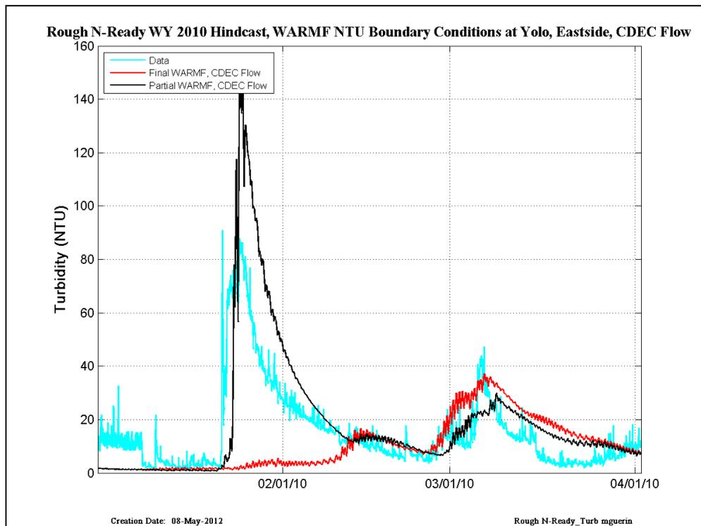
Figure 4 CDEC data (cyan) compared with RMA simulations run with Final WARMF (red) and Partial WARMF (black) – results are shown at Rough N'Ready Island on the San Joaquin River in WY2010.
