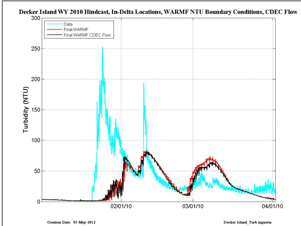
Figure 41 CDEC data (cyan) compared with RMA simulations run with Final WARMF (red) and Final WARMF and CDEC flows (black) – results are shown in Decker Island on the Sacramento River in WY2010.
