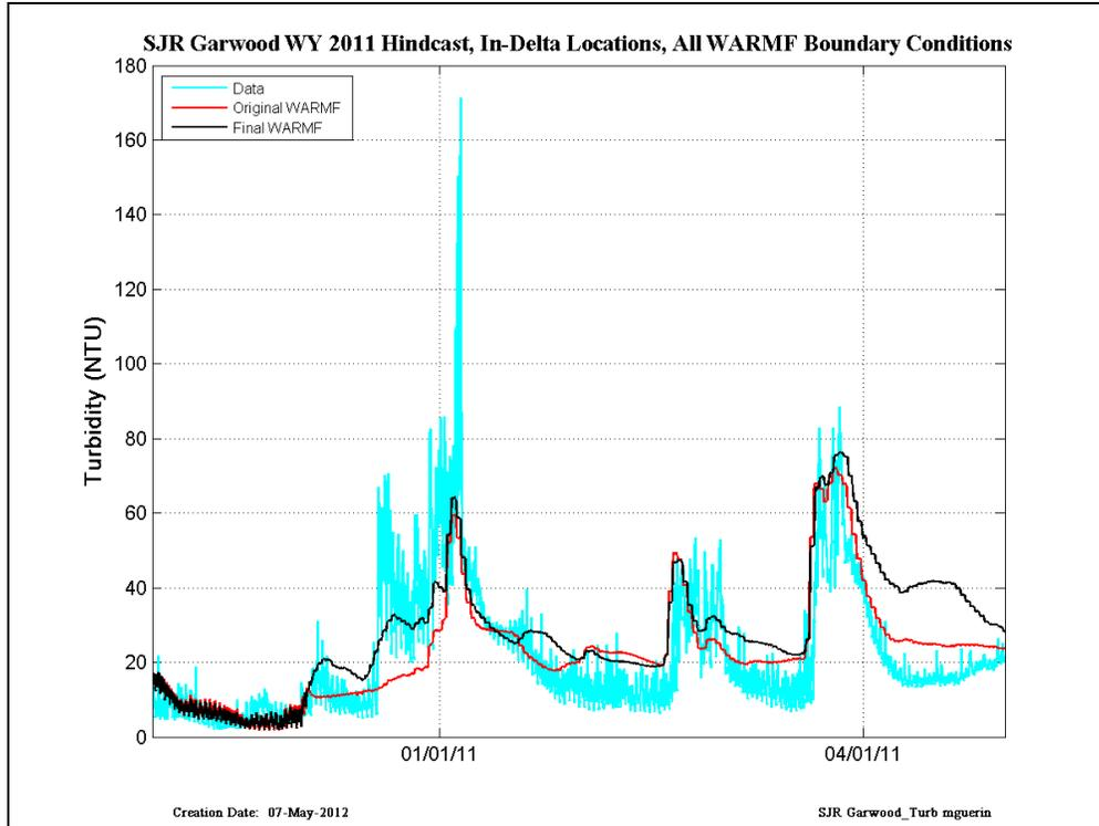
Figure 31 CDEC data (cyan) compared with RMA simulations run with original WARMF (red) and Final WARMF (black) – results are shown at SJR Garwood in WY2011.
