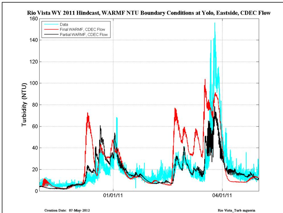
Figure 9 CDEC data (cyan) compared with RMA simulations run with Final WARMF (red) and Partial WARMF (black) – results are shown at Rio Vista in WY2011.
