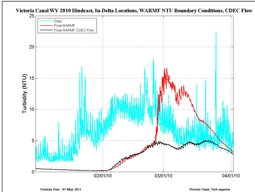
Figure 51 CDEC data (cyan) compared with RMA simulations run with Final WARMF (red) and Final WARMF and CDEC flows (black) – results are shown in Victoria Canal in WY2010.
