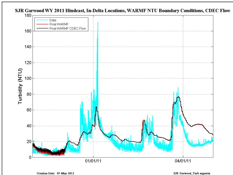
Figure 44 CDEC data (cyan) compared with RMA simulations run with Final WARMF (red) and Final WARMF and CDEC flows (black) – results are shown at Garwood on the San Joaquin River in WY2011.
