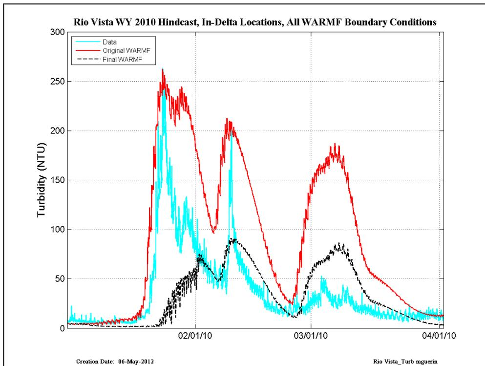
Figure 20 CDEC data (cyan) compared with RMA simulations run with original WARMF (red) and Final WARMF (black) – results are shown at Rio Vista in WY2010.
