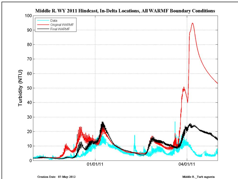
Figure 34 CDEC data (cyan) compared with RMA simulations run with original WARMF (red) and Final WARMF (black) – results are shown at Middle River in WY2011.
