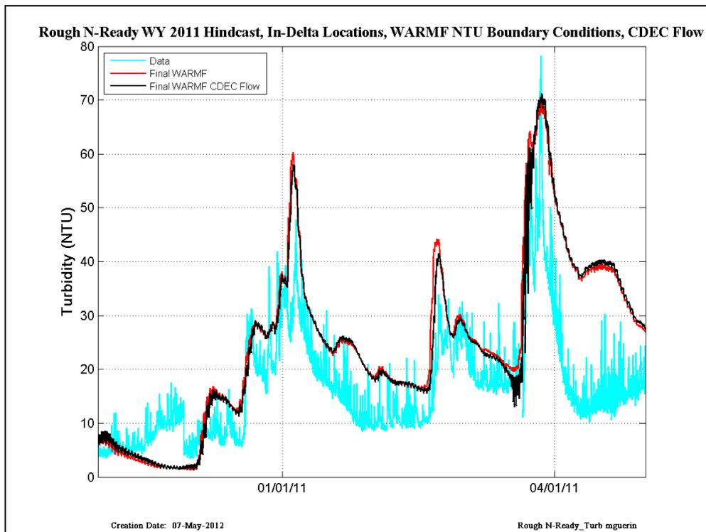
Figure 46 CDEC data (cyan) compared with RMA simulations run with Final WARMF (red) and Final WARMF and CDEC flows (black) – results are shown at Rough N’Ready on the San Joaquin River in WY2011.
