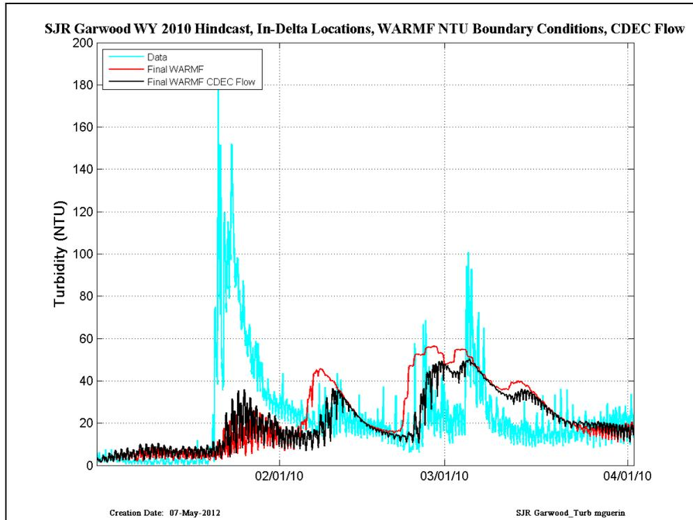
Figure 43 CDEC data (cyan) compared with RMA simulations run with Final WARMF (red) and Final WARMF and CDEC flows (black) – results are shown at Garwood on the San Joaquin River in WY2010.
