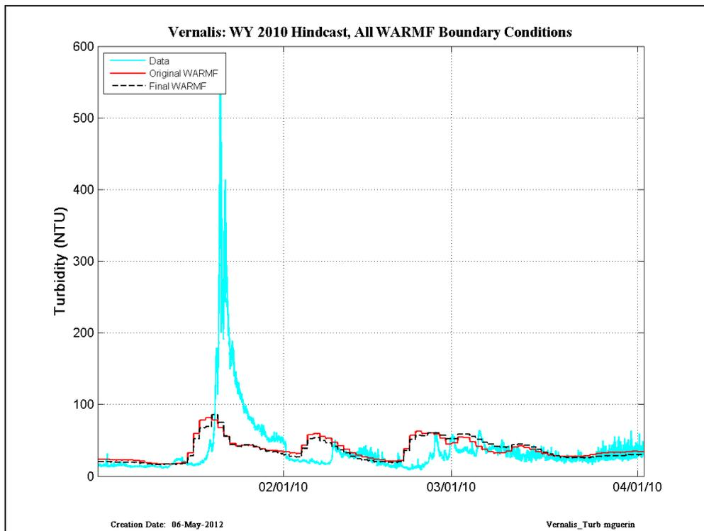
Figure 18 CDEC data (cyan) compared with RMA simulations run with original WARMF (red) and Final WARMF (black) – results are shown at Vernalis in WY2010.
