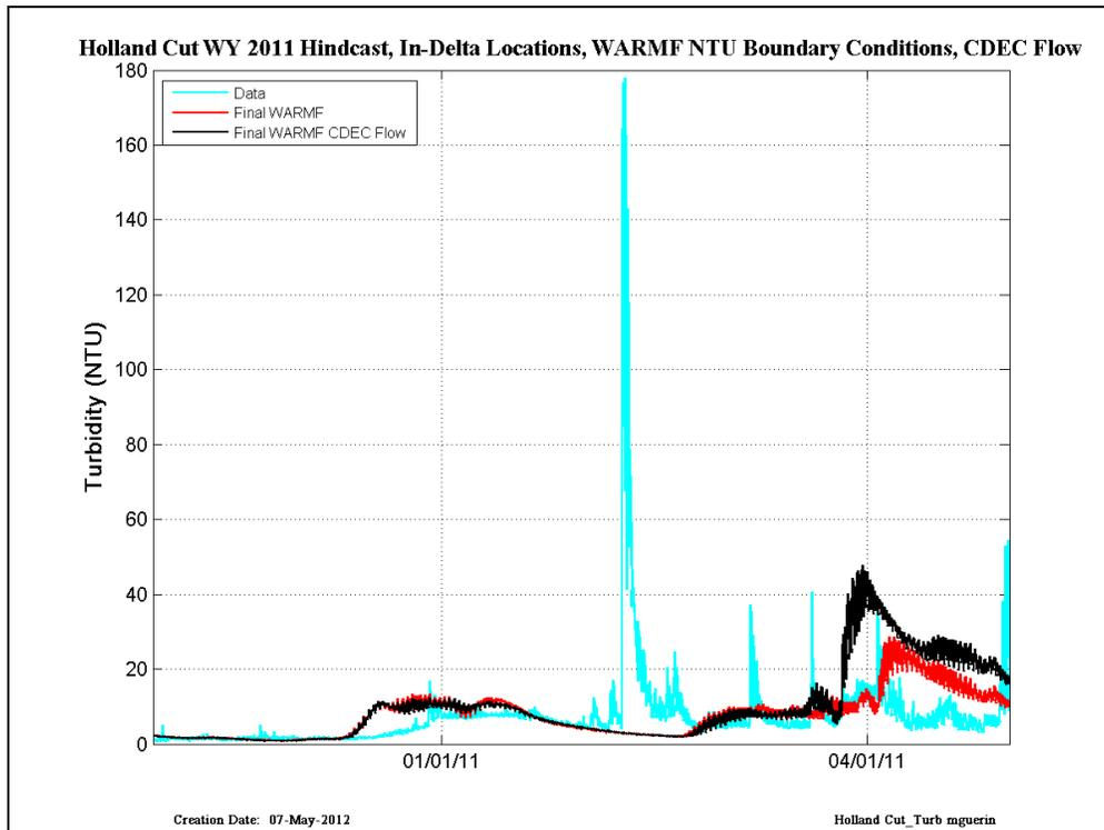
Figure 48 CDEC data (cyan) compared with RMA simulations run with Final WARMF (red) and Final WARMF and CDEC flows (black) – results are shown in Holland Cut in WY2011.
