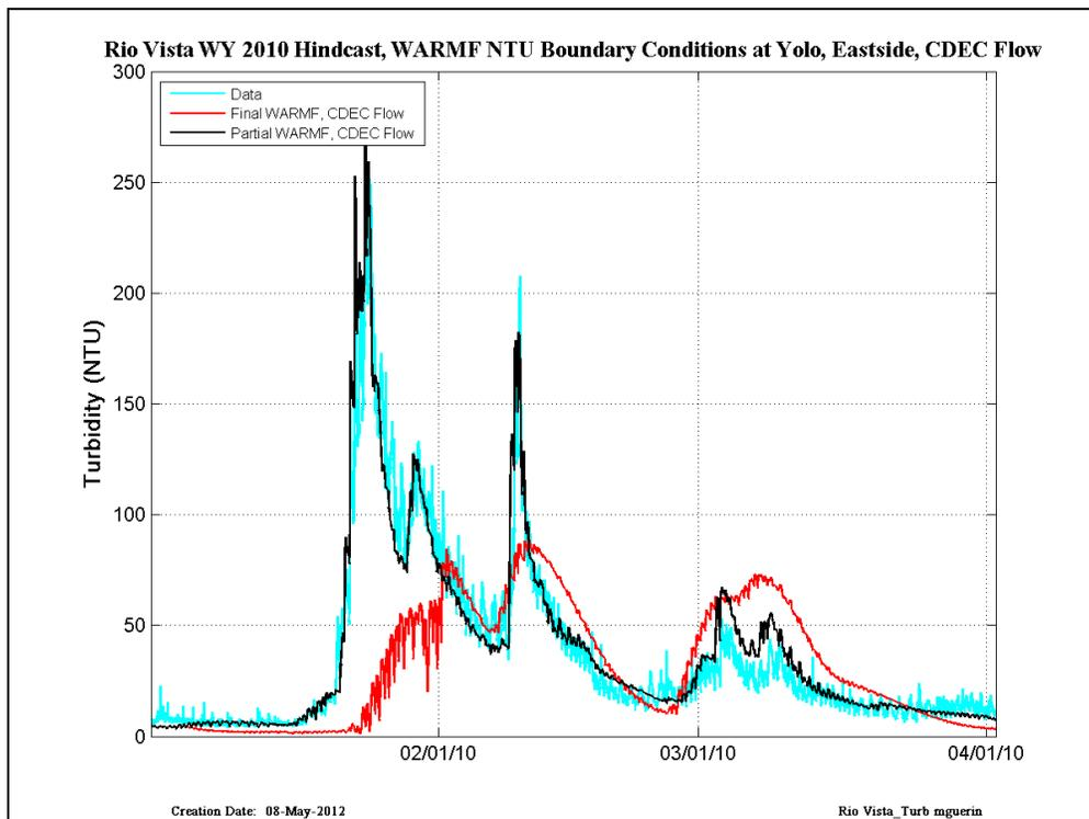
Figure 2 CDEC data (cyan) compared with RMA simulations run with Final WARMF (red) and Partial WARMF (black) – results are shown at Rio Vista in WY2010.
