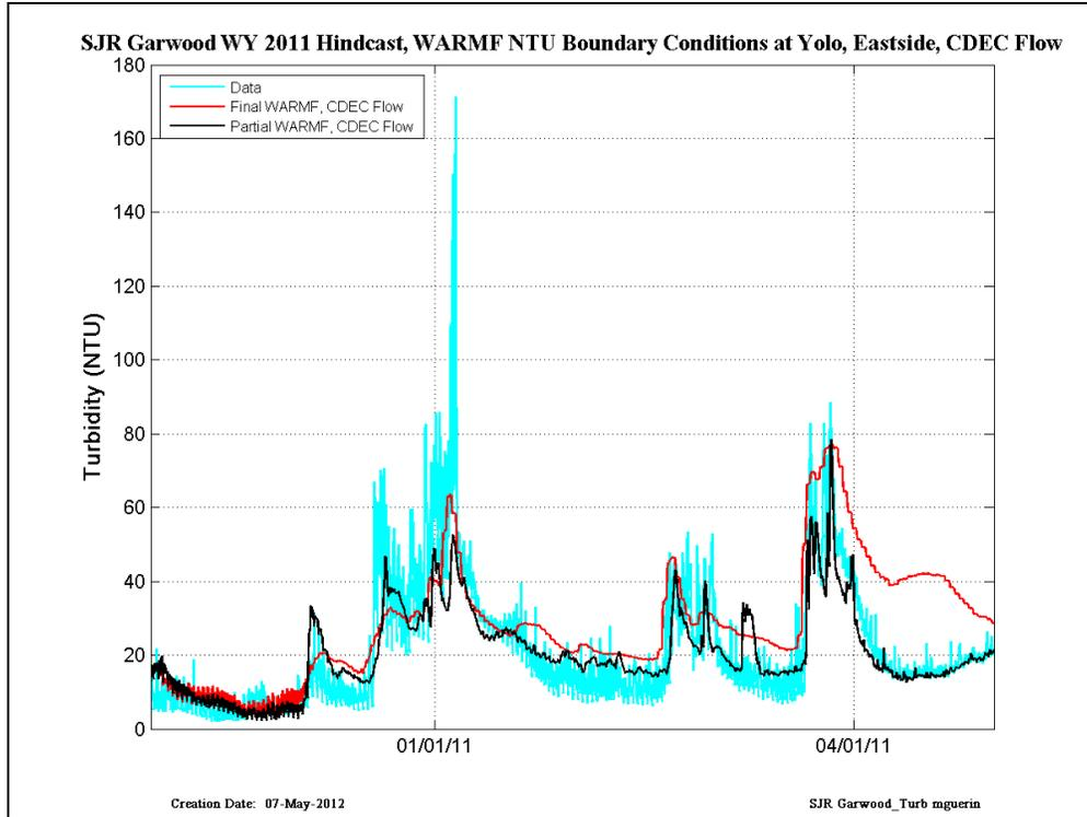
Figure 10 CDEC data (cyan) compared with RMA simulations run with Final WARMF (red) and Partial WARMF (black) – results are shown at Garwood on the San Joaquin River in WY2011.
