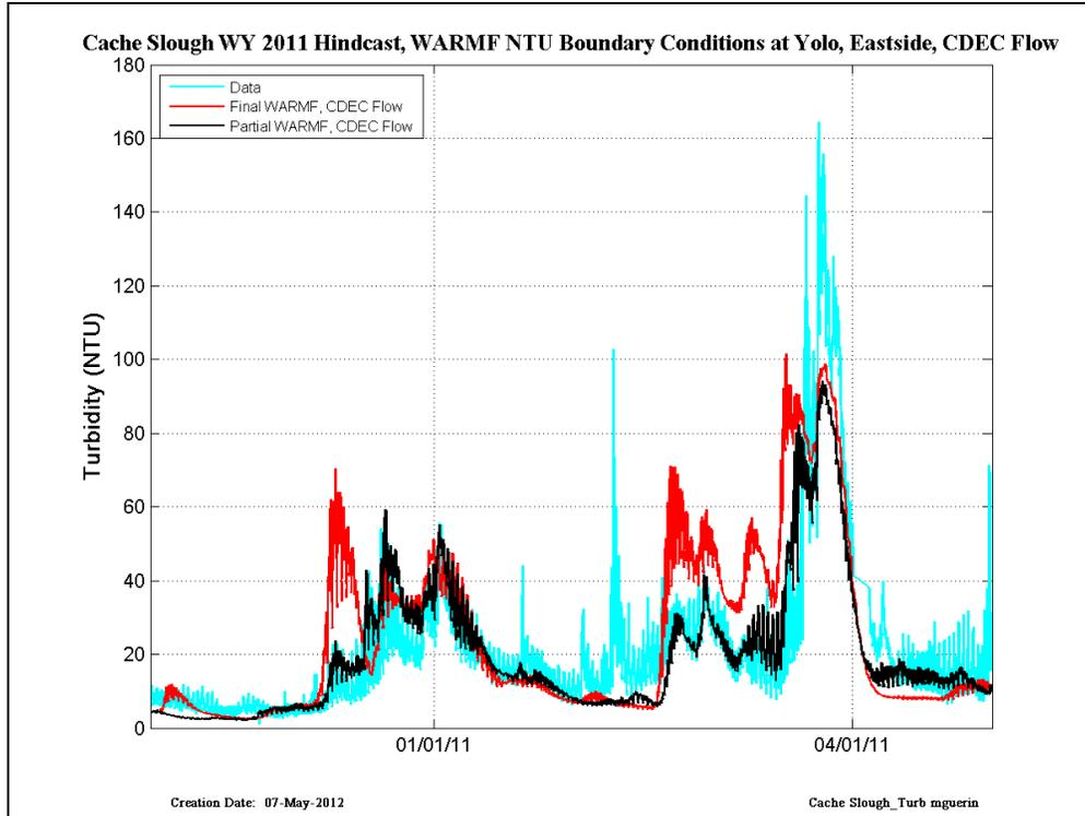
Figure 8 CDEC data (cyan) compared with RMA simulations run with Final WARMF (red) and Partial WARMF (black) – results are shown at Cache Slough at Ryer in WY2011.
