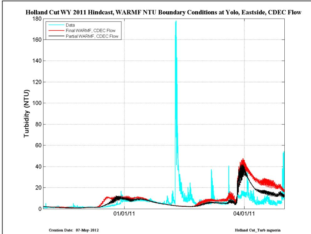
Figure 12 CDEC data (cyan) compared with RMA simulations run with Final WARMF (red) and Partial WARMF (black) – results are shown at Holland cut in WY2011.
