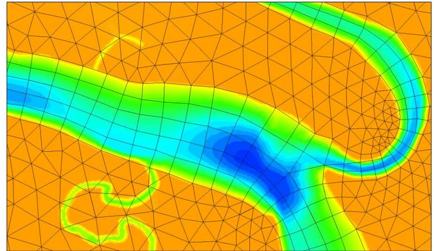
Model geometry with contoured subgrid bathymetry
