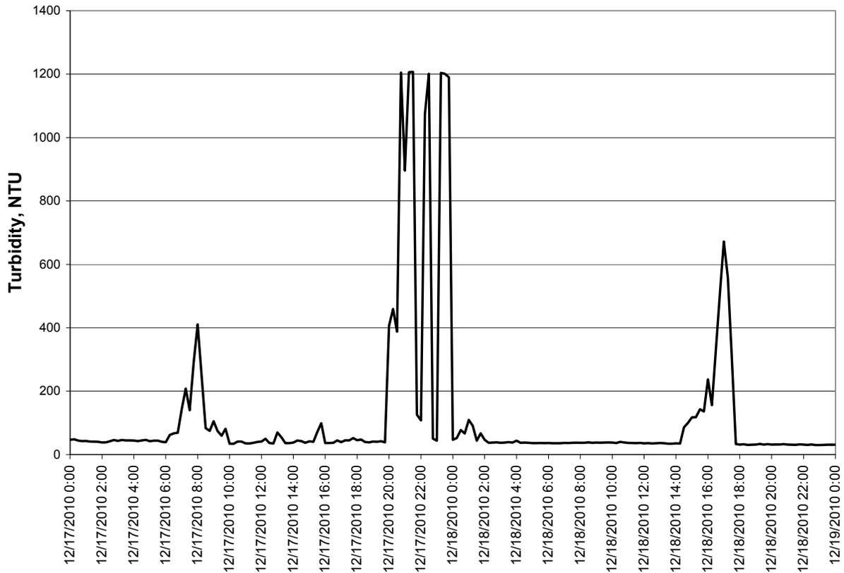
**Figure 4.8 Real-time Turbidity Measurement with Data Anomalies**
