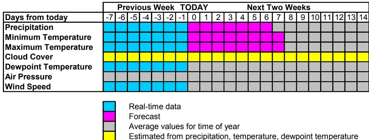
**Figure 2.3 Meteorology Data Sources for Real-time Hindcast and Forecast Simulations**
