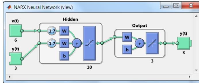
Figure 2-4 Matlab NARX ANN model structure ( $y(t) = f(x(t-1), \dots, x(t-d))$ ); inputs = 6 boundaries (3 flow + 3 turbidity), hidden neurons = 10; time delay = 1-7 days; outputs: turbidity at 3 locations). During training,  $y(t)$  on the left side can be approximated by the training data (termed “open loop”), and during testing,  $y(t)$  can be replaced by the ANN predicted value (termed “closed loop”).
