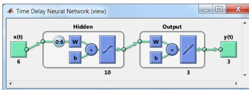
Figure 2-3 Feed-forward ANN model structure (inputs = 6 boundaries (3 flow + 3 turbidity), hidden neurons = 10; time delay = 7 days; outputs: turbidity at 3 locations).  $x(t)$  represents the input,  $y(t)$  the output, and  $W$  and  $b$  represents the weights and biases.
