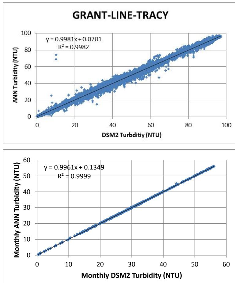
Figure D-30 DSM2 and ANN simulated turbidity at Grant Line Canal at Tracy (all data)
