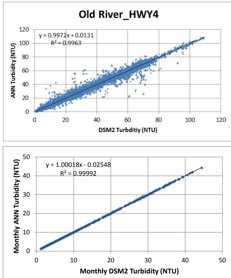
Figure D-22 DSM2 and ANN simulated turbidity at Old River at Highway 4 (all data)
