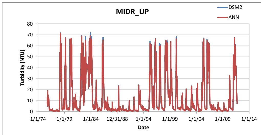
Figure D-27 DSM2 and ANN simulated turbidity at Middle River at Union Point (scenario 5)
