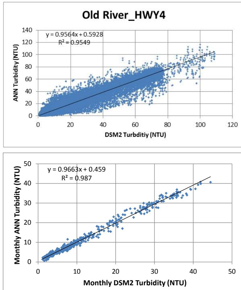
Figure C-22 DSM2 and ANN simulated turbidity at Old River at Highway 4 (all data)
