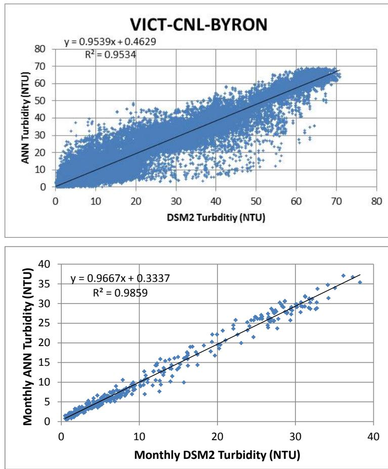
Figure C-26 DSM2 and ANN simulated turbidity at Victoria Canal (all data)
