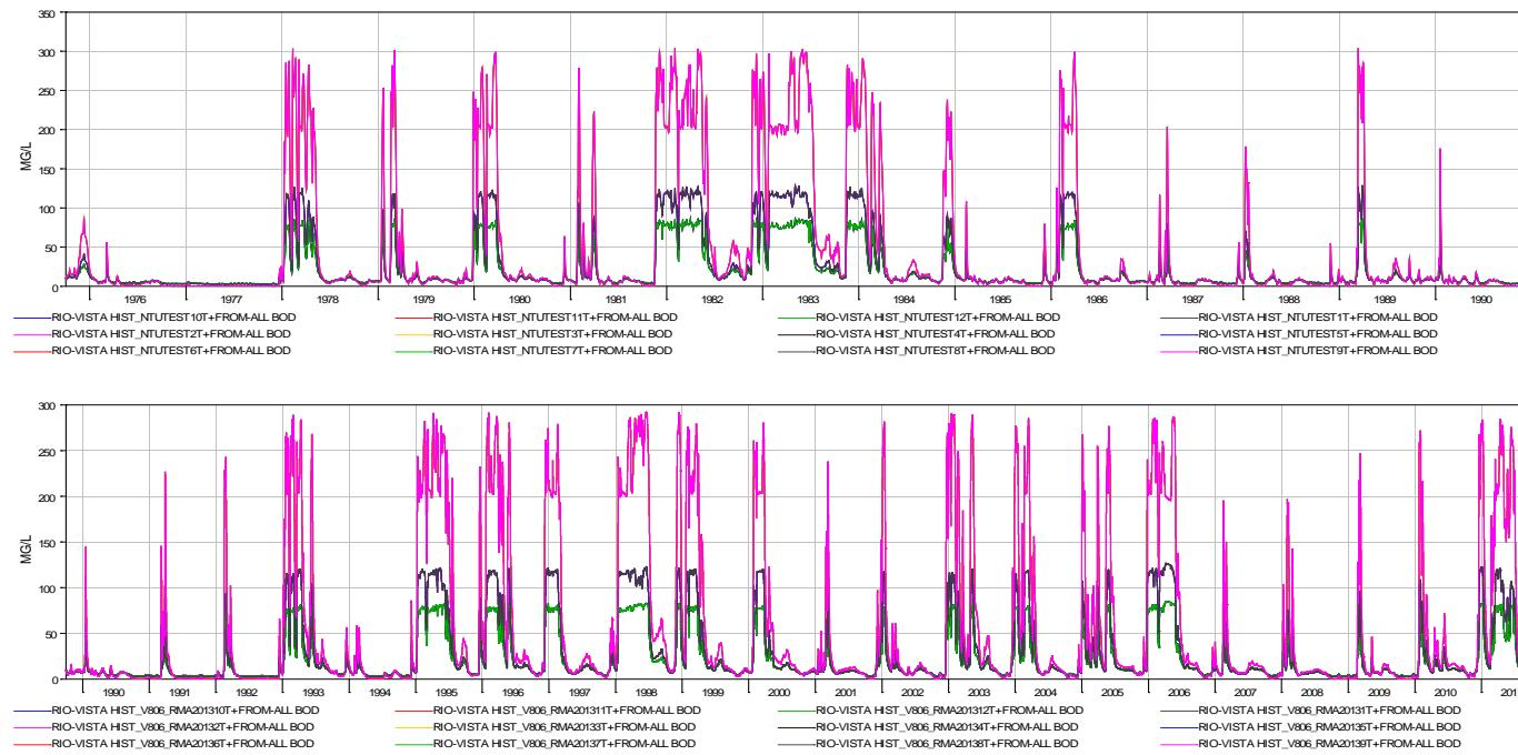
**Figure B-1** DSM2 simulated turbidity under twelve boundary conditions at Sacramento River at Rio Vista. Each line in this plot corresponds to a single boundary condition in Table 2-1.
