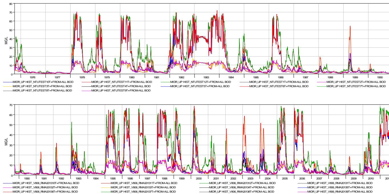
Figure B-14 DSM2 simulated turbidity under twelve boundary conditions at Middle River at Union Point
