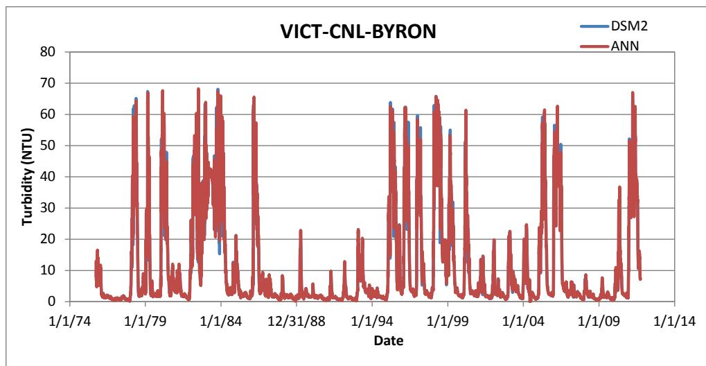
Figure D-25 DSM2 and ANN simulated turbidity at Victoria Canal (scenario 5)
