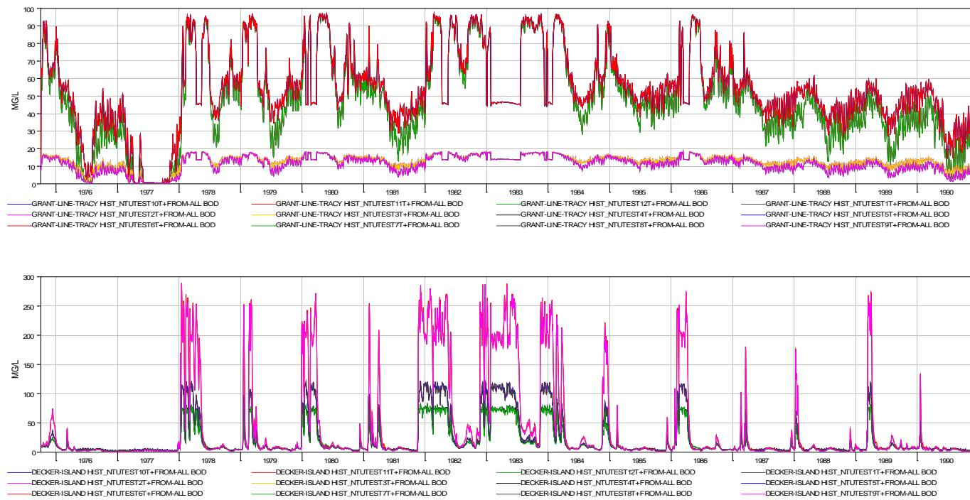
Figure B-2 DSM2 simulated turbidity under twelve boundary conditions at San Joaquin River at Decker Island
