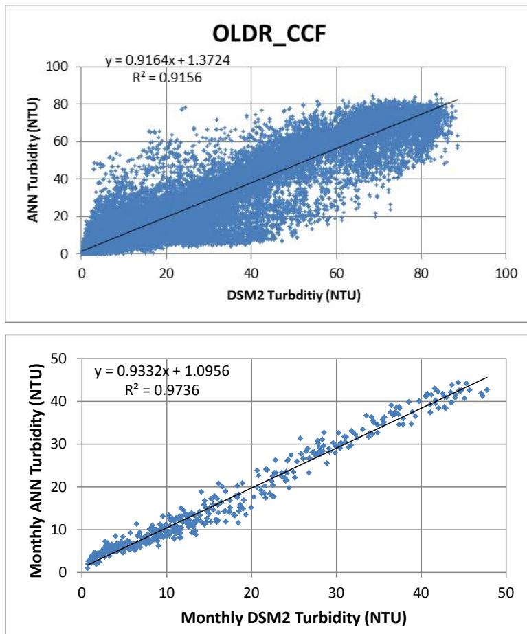
Figure C-24 DSM2 and ANN simulated turbidity at Old River at Clifton Court Intake (all data)
