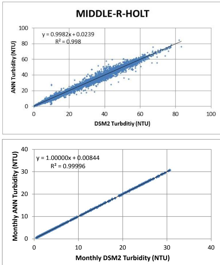
Figure D-16 DSM2 and ANN simulated turbidity at Middle River at Holt (all data)
