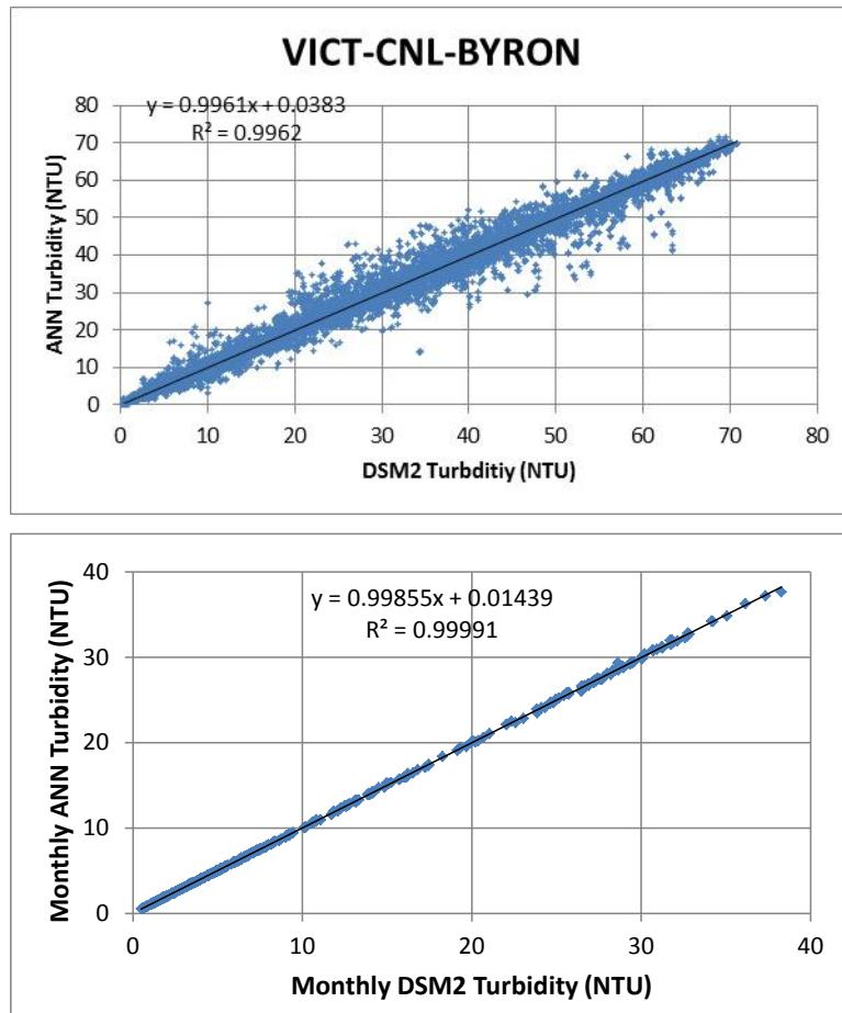
Figure D-26 DSM2 and ANN simulated turbidity at Victoria Canal (all data)
