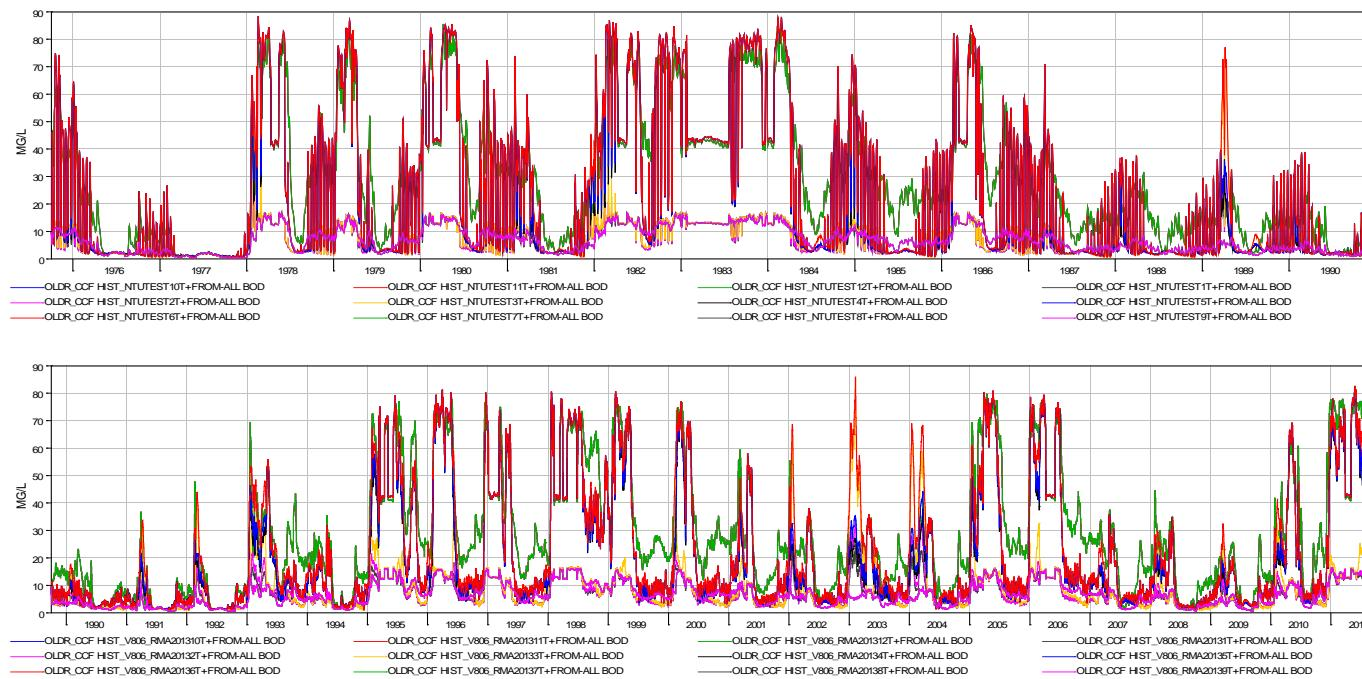
Figure B-12 DSM2 simulated turbidity under twelve boundary conditions at Old River at Clifton Court Intake
