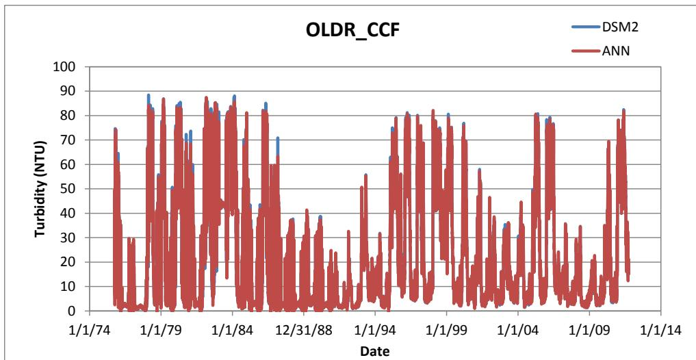
Figure D-23 DSM2 and ANN simulated turbidity at Old River at Clifton Court Intake (scenario 5)
