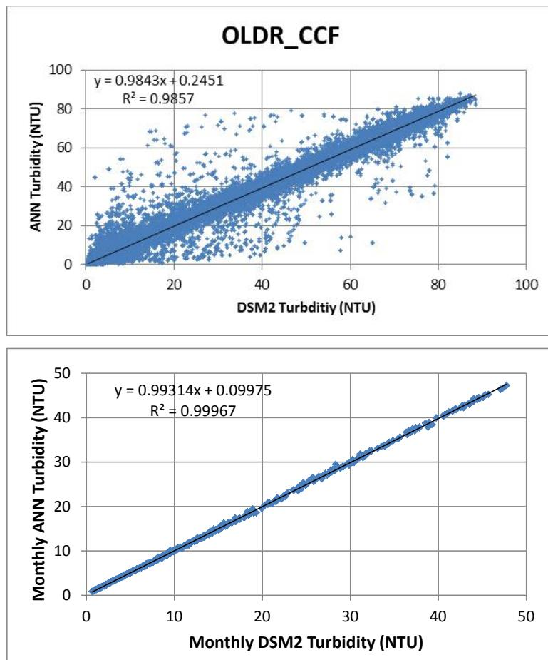
Figure D-24 DSM2 and ANN simulated turbidity at Old River at Clifton Court Intake (all data)
