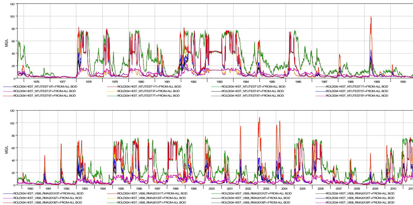
Figure B-11 DSM2 simulated turbidity under twelve boundary conditions at Old River at Hwy 4
