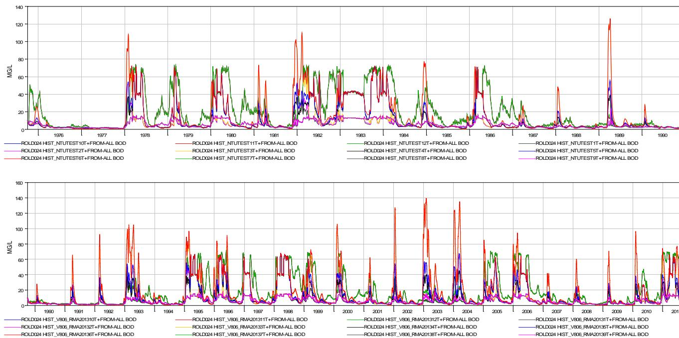
Figure B-7 DSM2 simulated turbidity under twelve boundary conditions at Old River at Bacon Island
