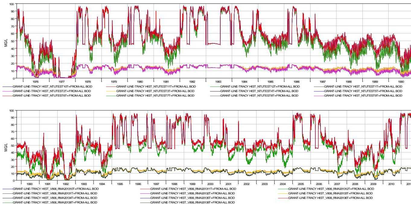
*Figure B-15 DSM2 simulated turbidity under twelve boundary conditions at Grant Line Canal at Tracy*
