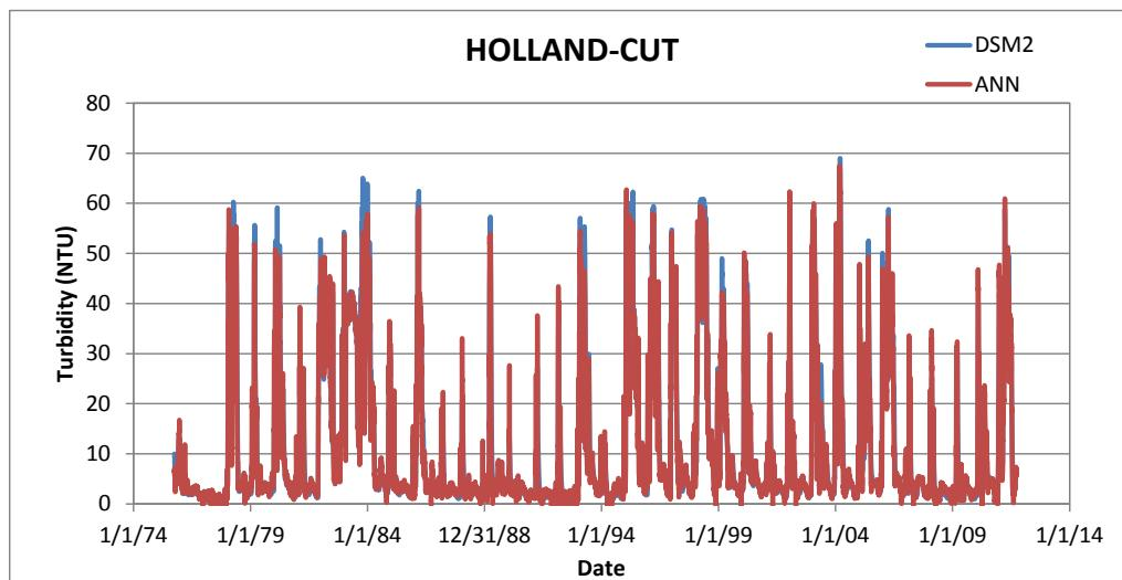
Figure C-9 DSM2 and ANN simulated turbidity at Old River @ Holland Cut (scenario 5)
