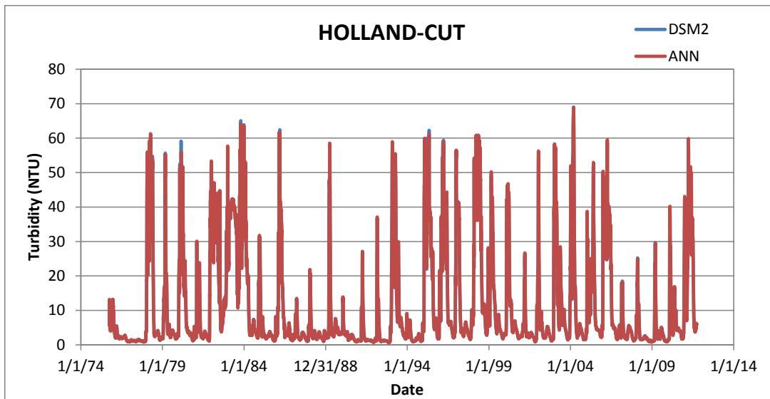
Figure D-9 DSM2 and ANN simulated turbidity at Old River @ Holland Cut (scenario 5)
