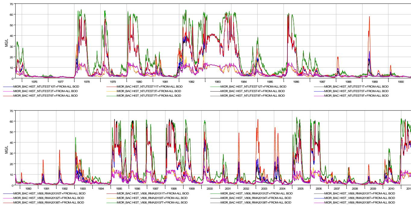
Figure B-9 DSM2 simulated turbidity under twelve boundary conditions at Middle River at Bacon Island
