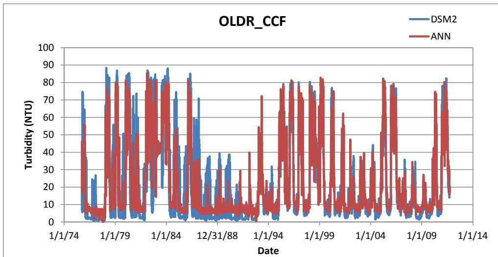
Figure C-23 DSM2 and ANN simulated turbidity at Old River at Clifton Court Intake (scenario 5)
