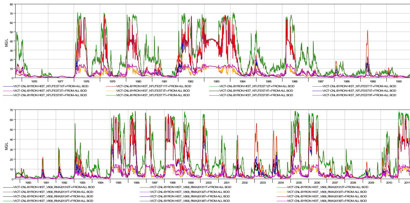
Figure B-13 DSM2 simulated turbidity under twelve boundary conditions at Victoria Canal
