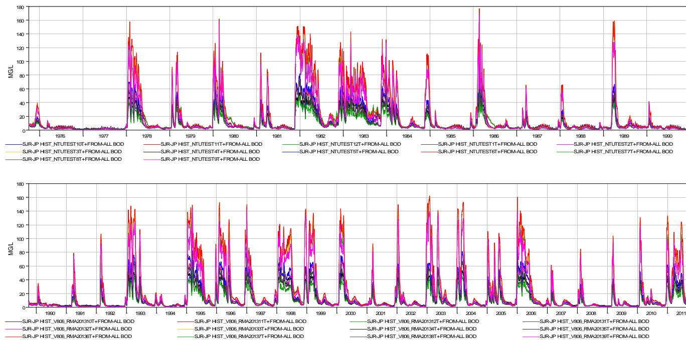
Figure B-3 DSM2 simulated turbidity under twelve boundary conditions at San Joaquin River at Jersey Point
