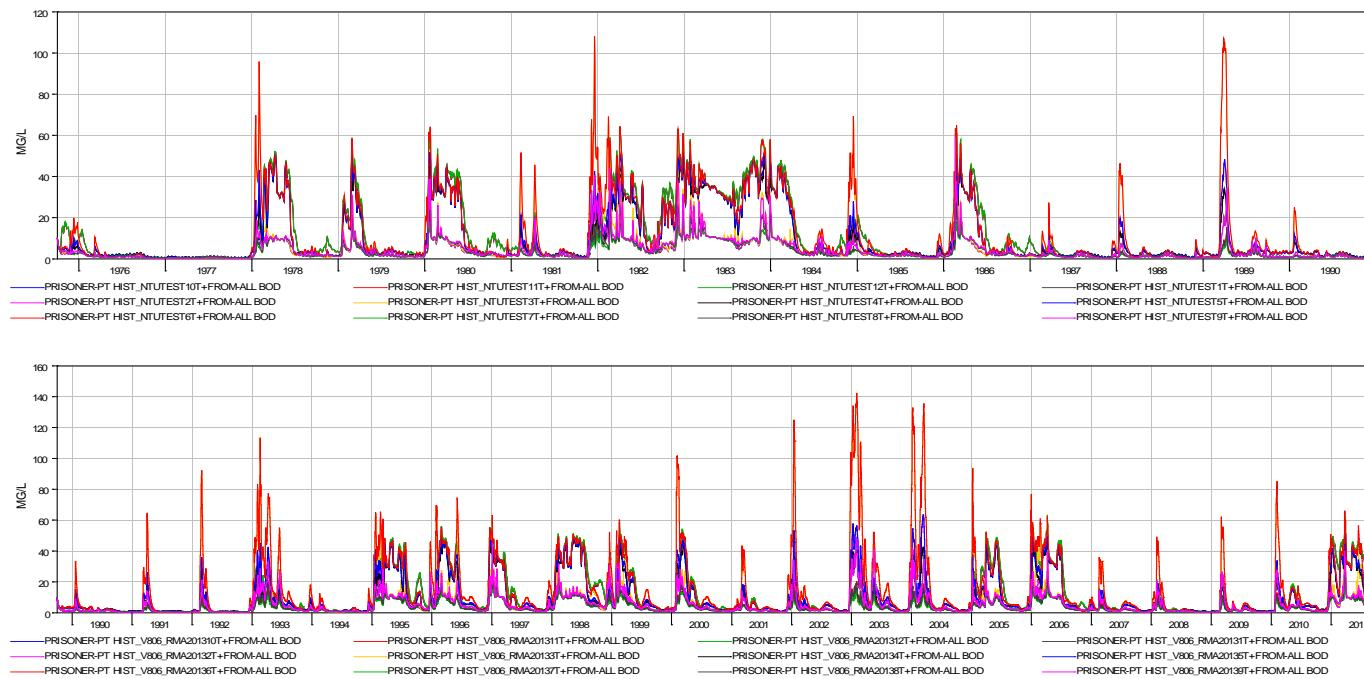
Figure B-4 DSM2 simulated turbidity under twelve boundary conditions at San Joaquin River at Prisoner's Point
