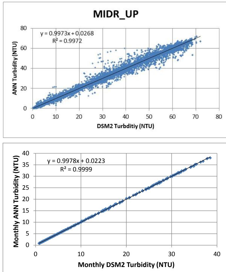
Figure D-28 DSM2 and ANN simulated turbidity at Middle River at Union Point (all data)
