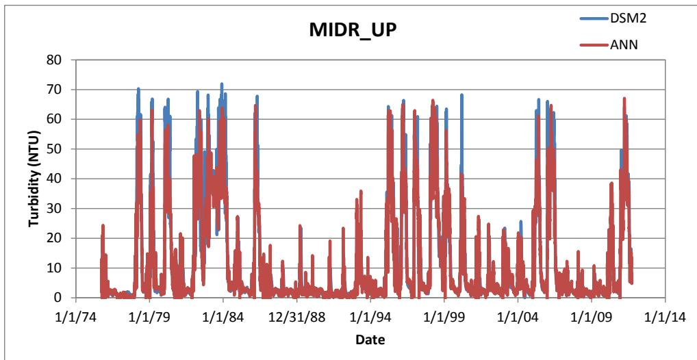
Figure C-27 DSM2 and ANN simulated turbidity at Middle River at Union Point (scenario 5)
