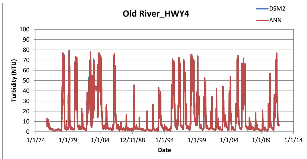
Figure D-21 DSM2 and ANN simulated turbidity at Old River at Highway 4 (scenario 5)
