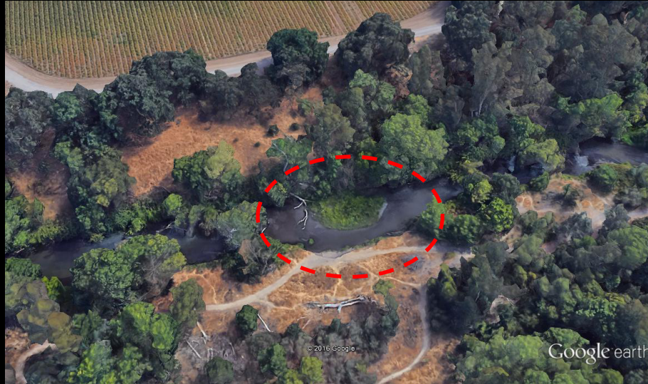
Island and point bar evolution on Putah Creek break up oversized bathtub sections
