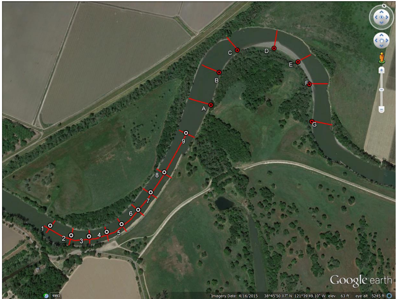
Figure 25 - Location of the proposed 2016 study secondary circulation transect locations (transects 1-6) associated with the 2D-array. Collecting secondary circulation in the 180 degree oxbow at transects A-G are also proposed, if time allows. Understanding the transition of secondary circulation from a 90 deg bend (transects 1-7) immediately into the 180 deg bend will be useful in determining the spatial scales of secondary circulation initiation, peak and relaxation and as a validation data set for numerical models of the region.
