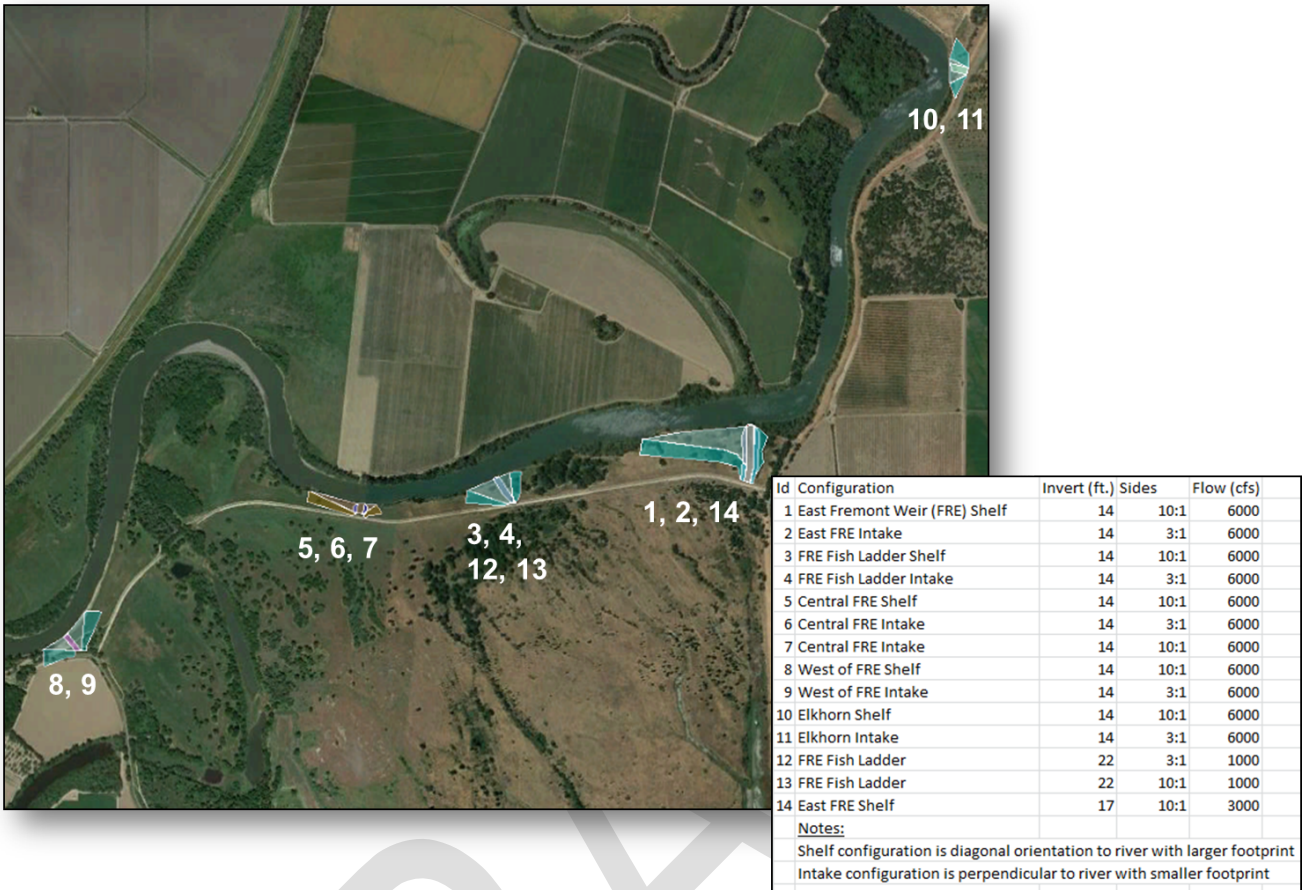
Figure 13 - Location of the Fremont Weir notch alternatives that are currently being modeled in ELAM. These notch alternative locations were considered for the placement of a coarse telemetry array aimed at documenting baseline spatial distributions at these locations. Figure prepared by Joshua Urias (DWR) on 12/18/15 for Jon Burau (USGS).
