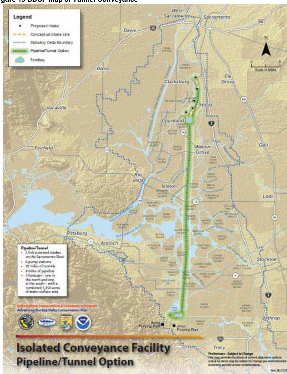
Figure 19 BDCP Map of Tunnel Conveyance 93
