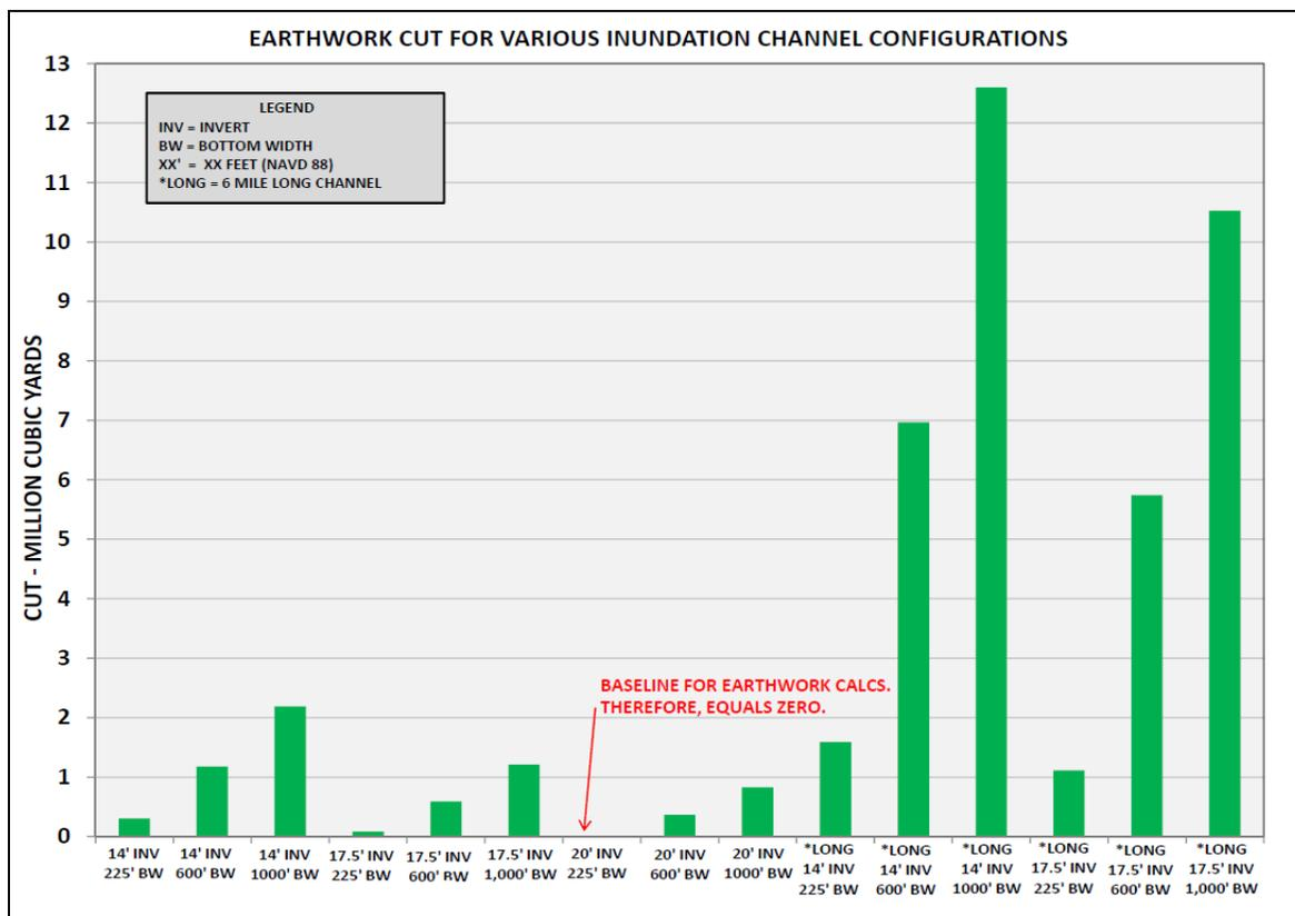
**Figure C.5. Earthwork Cut for Various Inundation Channel Configurations**
