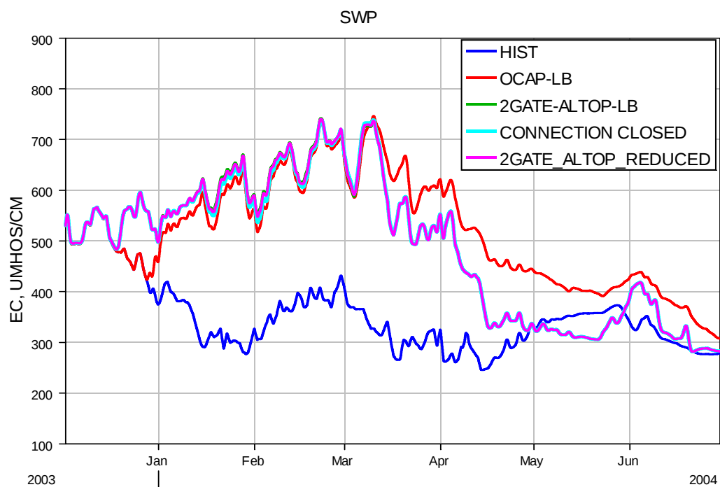
Figure 19 Tidally averaged EC at the SWP for the 2003-2004 simulation period for HIST, OCAP-LB and 2GATE-ALTOP-LB, CONNECTION CLOSED and 2GATE_ALTOP_REDUCED simulations.
