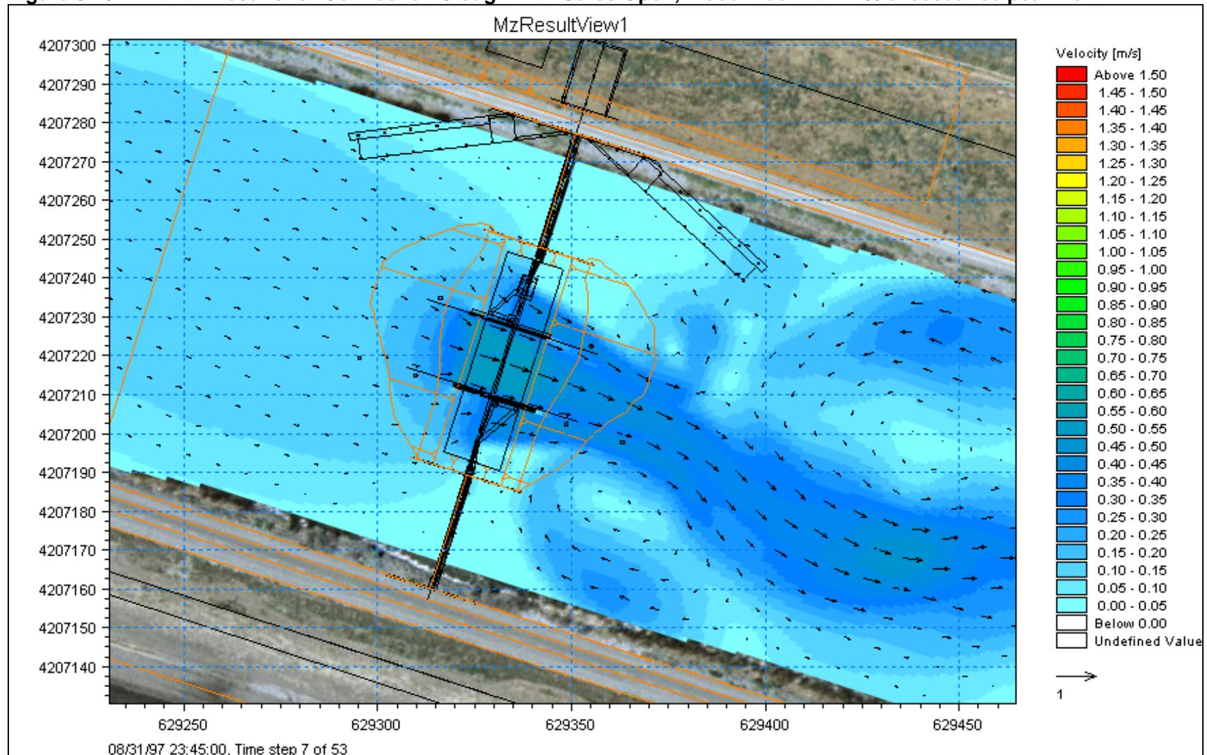
Figure 3.11 MIKE-21 Results for Connection Slough with Gates Open, Ebb Tide ~1% exceedance peak flow.
