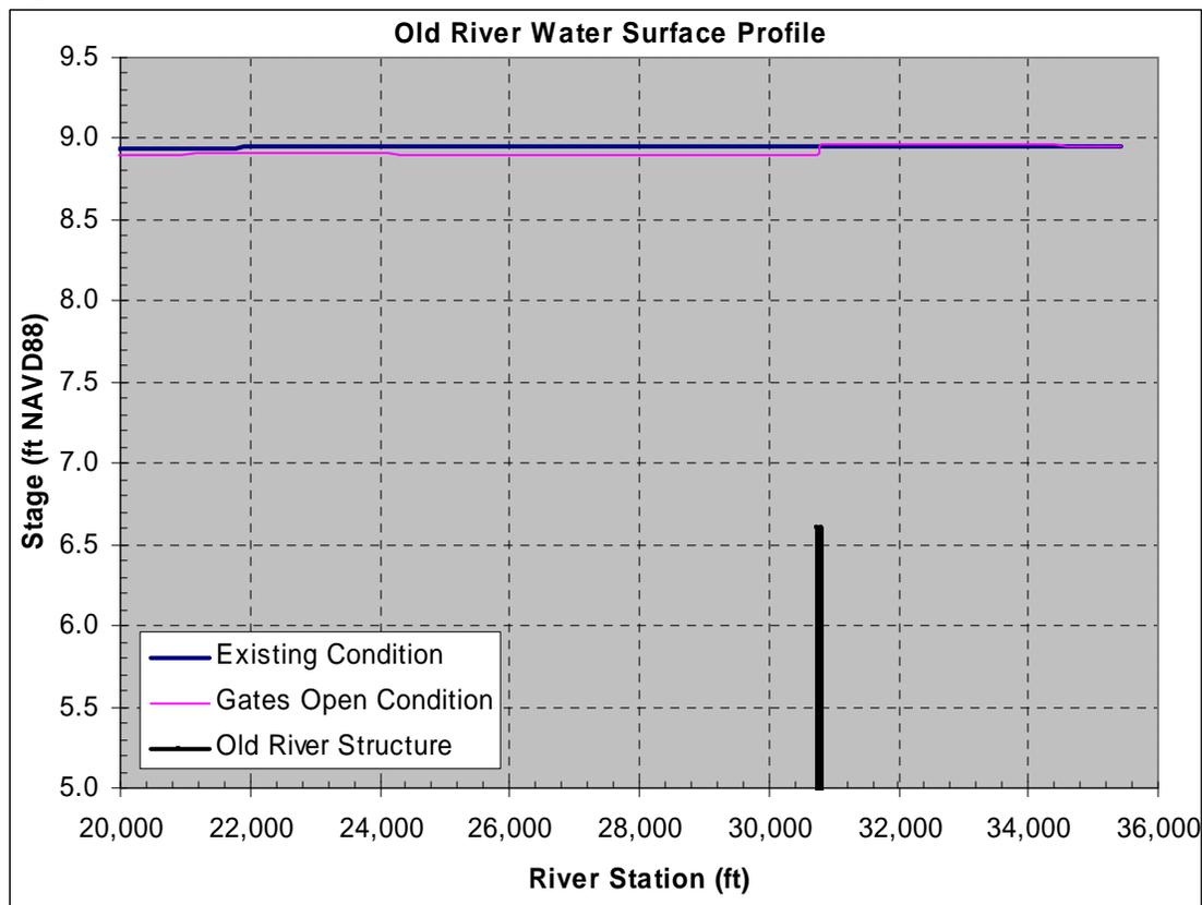
Figure 3.7 MIKE-21 Results for Old River with Gates Open, Flood Tide with ~0.02% exceedance peak flow.
