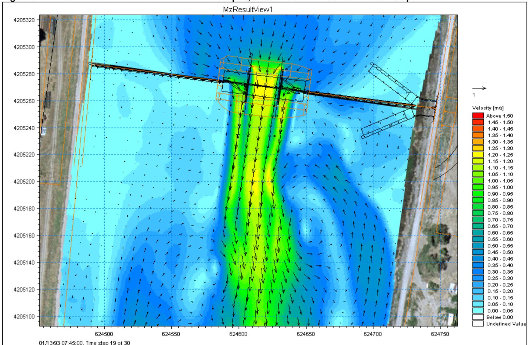
Figure 3.8 MIKE-21 Results for Old River with Gates Open, Flood Tide with ~1% exceedance peak flow.
