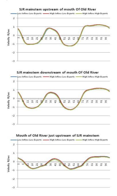
Figure 3-8. DSM2 Modeled Instantaneous 15-Minute Velocity Versus Time Over a Complete Tidal Cycle (~25 Hours) in Three Channels at the Junction of the San Joaquin River Mainstem and the Mouth of Old River
