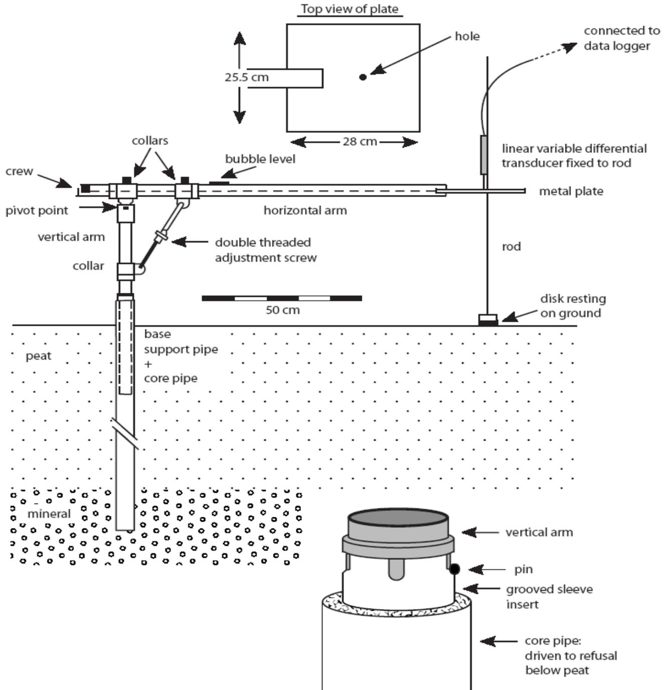
**Figure 10. Extensometer in rice field.**
