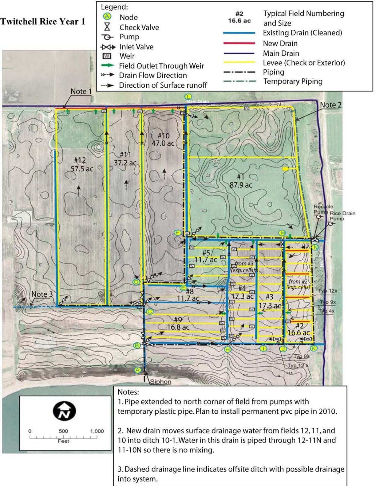
**Figure 4. Water delivery and drainage system.**
