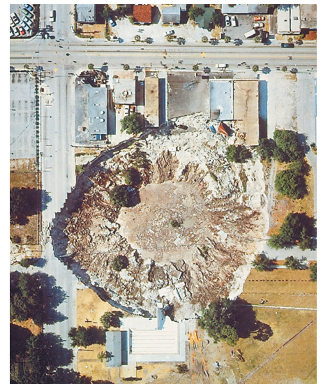
Figure 8. Collapse sinkholes, such as this one in Winter Park, Florida (1981), may develop abruptly (over a period of hours) and cause catastrophic damage.
