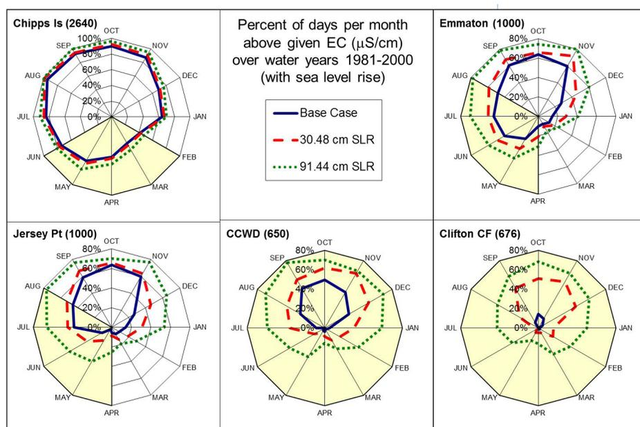
**Figure 9** Simulated percentage of days each month exceeding the specified EC ( $\mu\text{S cm}^{-1}$ ) at locations in the Delta with sea level rise. The figure shows the average monthly values over the simulation period 1981–2000, with 1981–2000 levels of upstream reservoir operations and Delta exports. Shaded areas are periods when compliance with salinity standards is prescribed, although compliance levels vary across water year types (and across months for irrigation standards).
