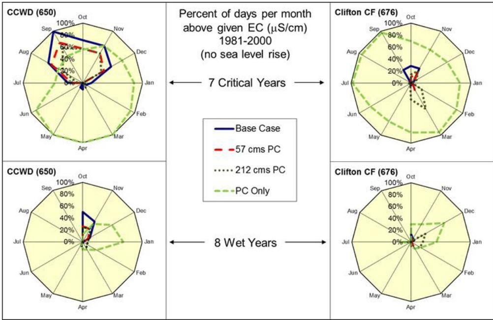
**Figure 14** Comparison of wet and critical water years with simulated average percentage of days in each month exceeding the specified EC ( $\mu\text{S cm}^{-1}$ ) at the CCWD pumping plant and Clifton Court Forebay. Shaded areas are periods when compliance with salinity standards is prescribed, although compliance levels vary across water year types. Drinking water standard is all 12 months.
