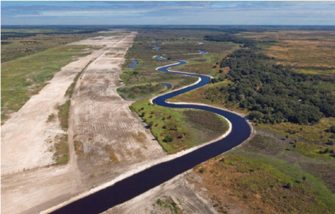
Kissimmee River restoration, showing flood control channel filled in so river meanders could be restored.
