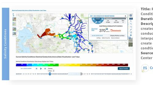
Title: Real-Time Salinity **Conditions Visualization Duration:** Last 7 Days Description: Salinity model created from real-time electrical conductivity station data, interpolated and transformed to create color gradients of salinity condtions throughout the Delta. Source: California Data Exchange
