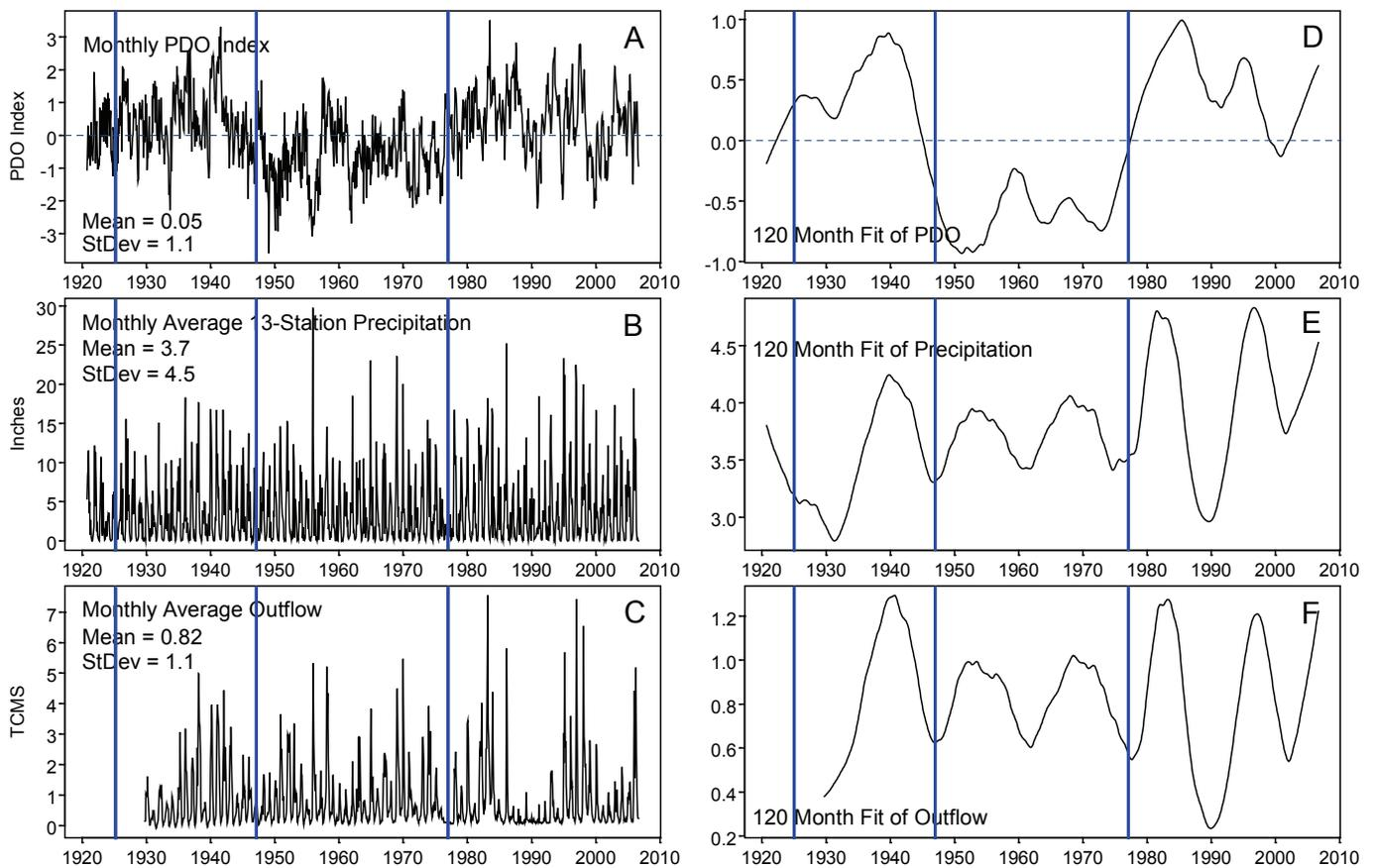
**Figure 7** Left column (A, B, C) shows PDO, 13-station precipitation and outflow time-series. Right hand column (D, E, F) shows 120-month loess fits to the data to highlight possible correlation between “decadal” scale variability in PDO and precipitation and outflow. Blue verticals indicate PDO polarity shift.
