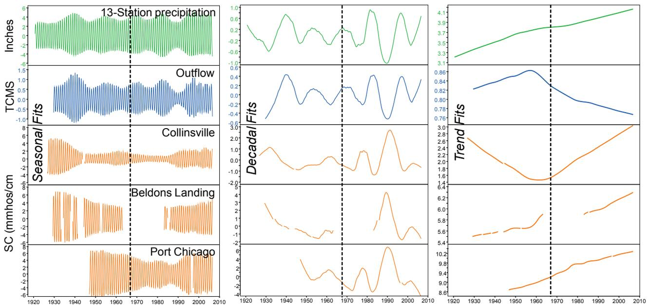
**Figure 5** Seasonal loess trend decomposition on monthly average 13-station precipitation, outflow, and salinity data. Right column is the “seasonal” fit based on a 12-month frequency mode. Middle column is the 120 month “decadal” fit of the seasonal fit residuals. Right column is the “trend” fit to the decadal fit residuals. Dotted vertical lines delineate “pre” and “post” project periods.
