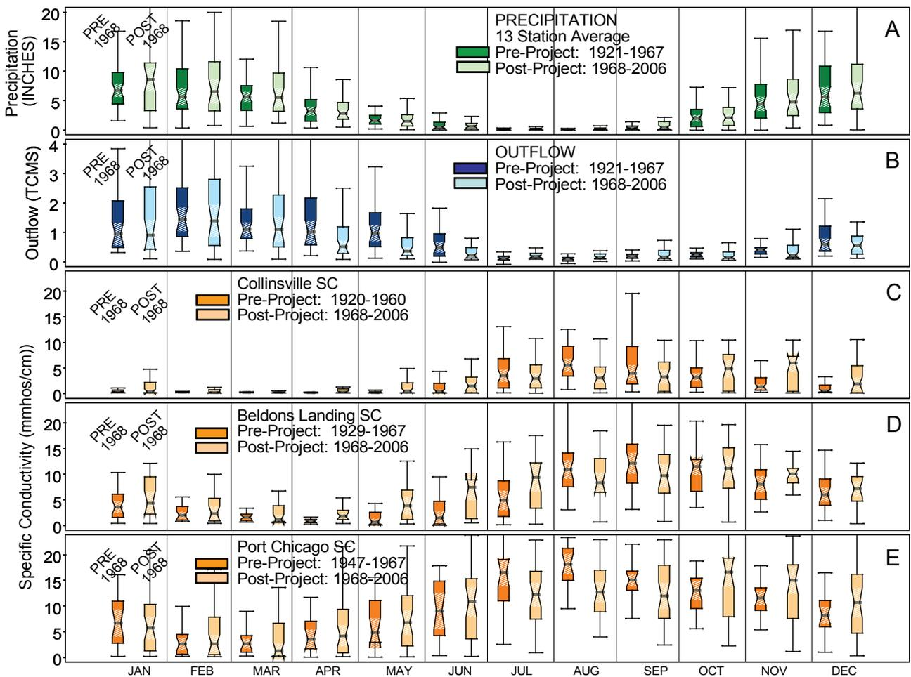
**Figure 14** Distribution of pre- and post-project precipitation, outflow, and salinity by month. Box-plot indicates median, 95% confidence interval, inner quartile, and range of data for each month. Pre-project and post-project distributions are shown side-by-side for each month.
