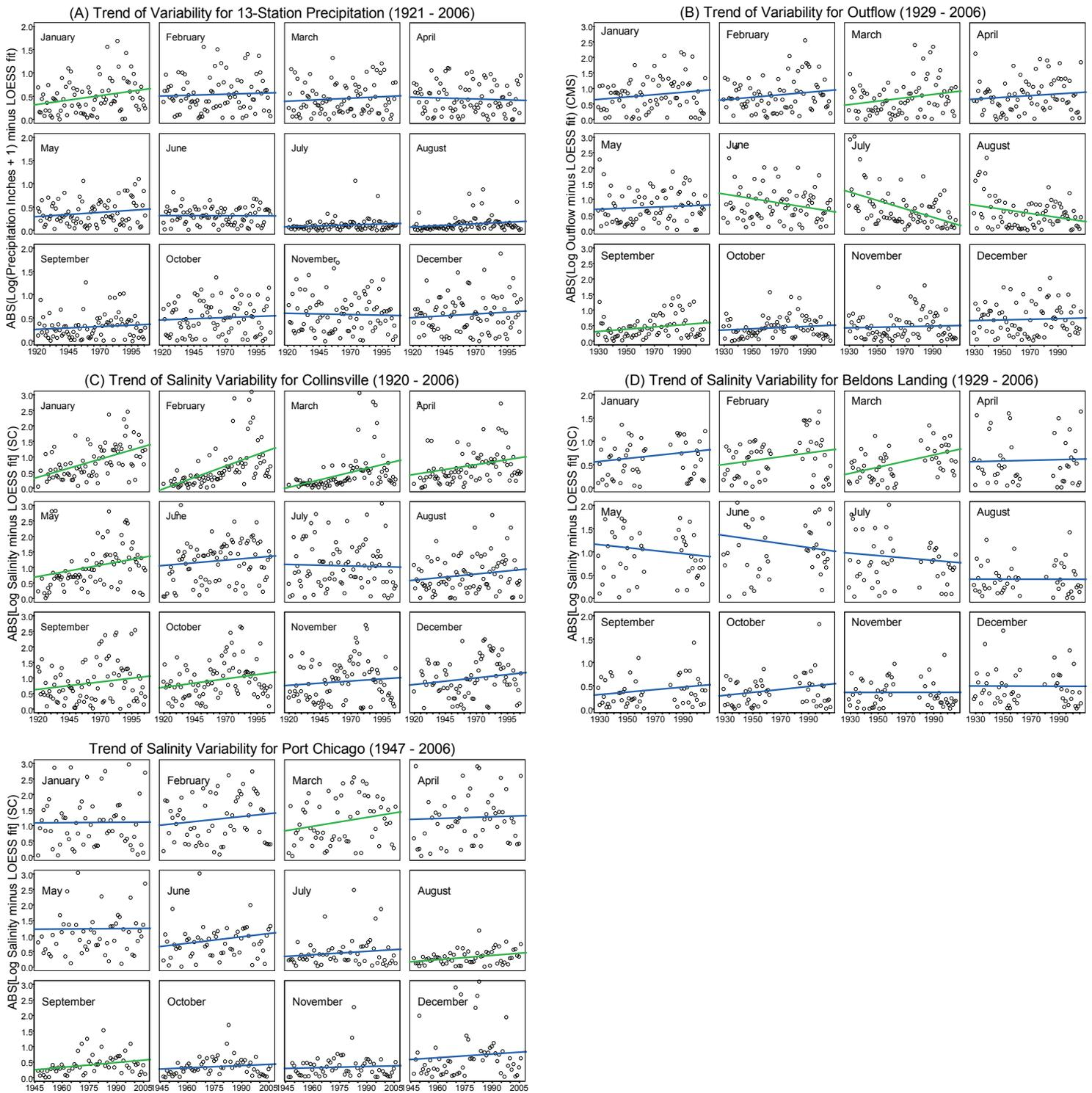
**Figure 13** Trend of variability based on local regression fits to the average of 13 Bay-Delta watershed precipitation stations by month. Circles are absolute value of data residuals minus loess fit. Lines are regression fits. Green regression fits indicate significant slopes ( $p < 0.05$ ) suggesting trend in variability. Blue is not significant.
