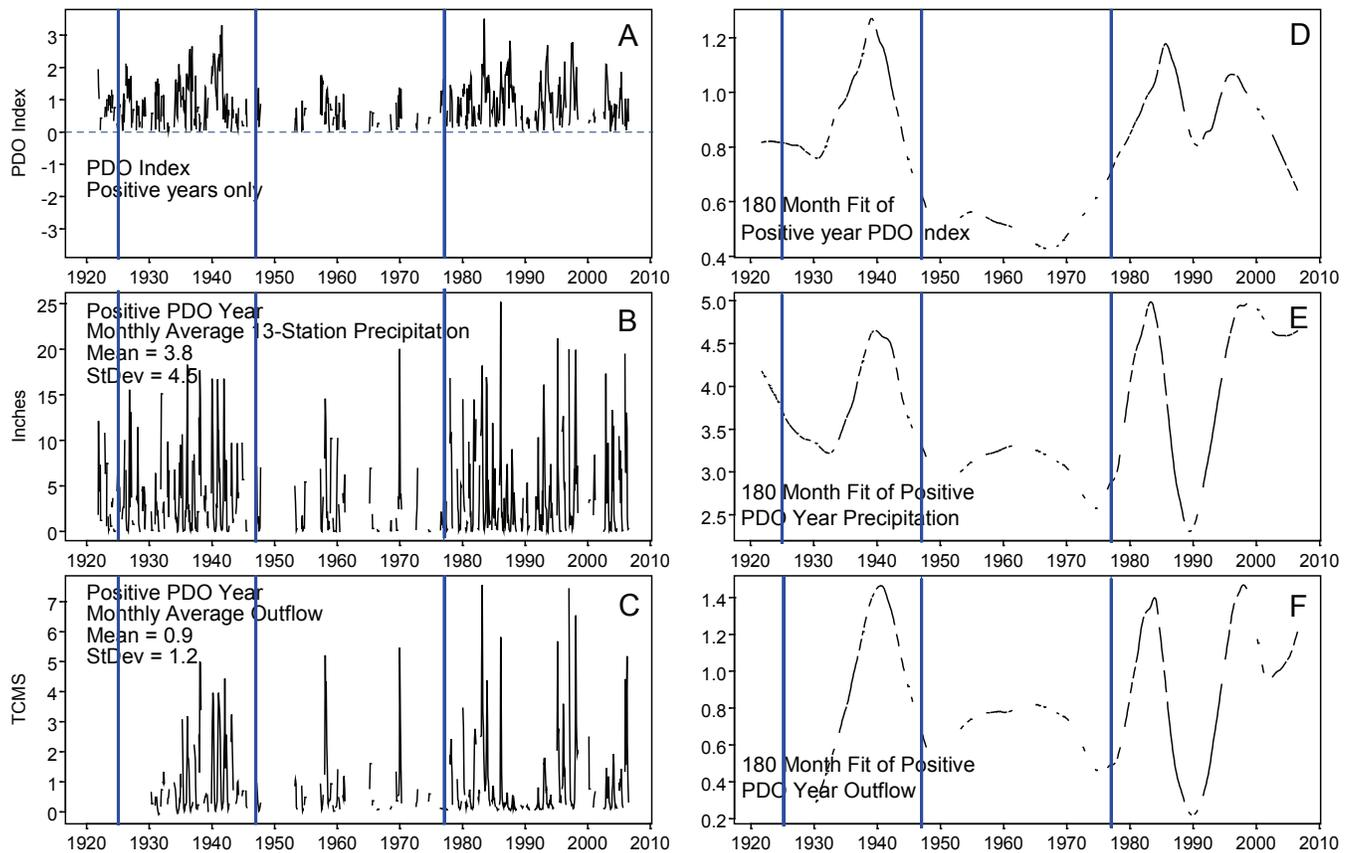
**Figure 8** Left column (A, B, C) shows positive polarity PDO years only with corresponding 13-station precipitation and outflow time-series. Right hand column (D, E, F) shows 180 month loess fits to the data to highlight possible correlation between "decadal" scale variability in positive PDO years and same timescale precipitation and outflow. Blue verticals indicate PDO polarity shift.
