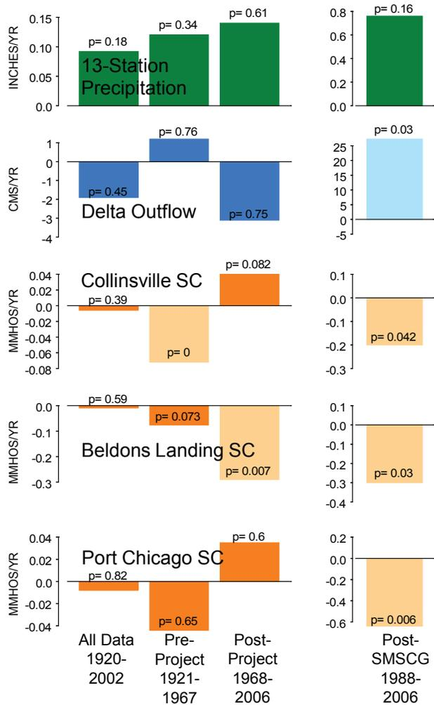
**Figure 10** Slope of trend in annual data by Kendall's test. Annual data binned as all data, pre-project, post-project, and post SMSCG. Note SC is plotted on different y-axis scales. All post-SMSCG data is plotted on a different y-axis scale. Pastel bars are significant.
