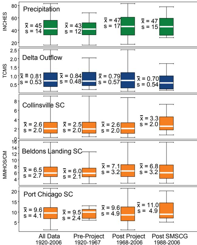
**Figure 4** Box and whisker plot of annual average statistics for 13-station precipitation, outflow and SC data. Data is binned as 1) all data, 2) pre-project (prior to 1968), 3) post project (after 1968), and post SMSCG (after 1988) periods. Box is inner quartiles, line is median. The mean and standard deviation are posted aside each box.
