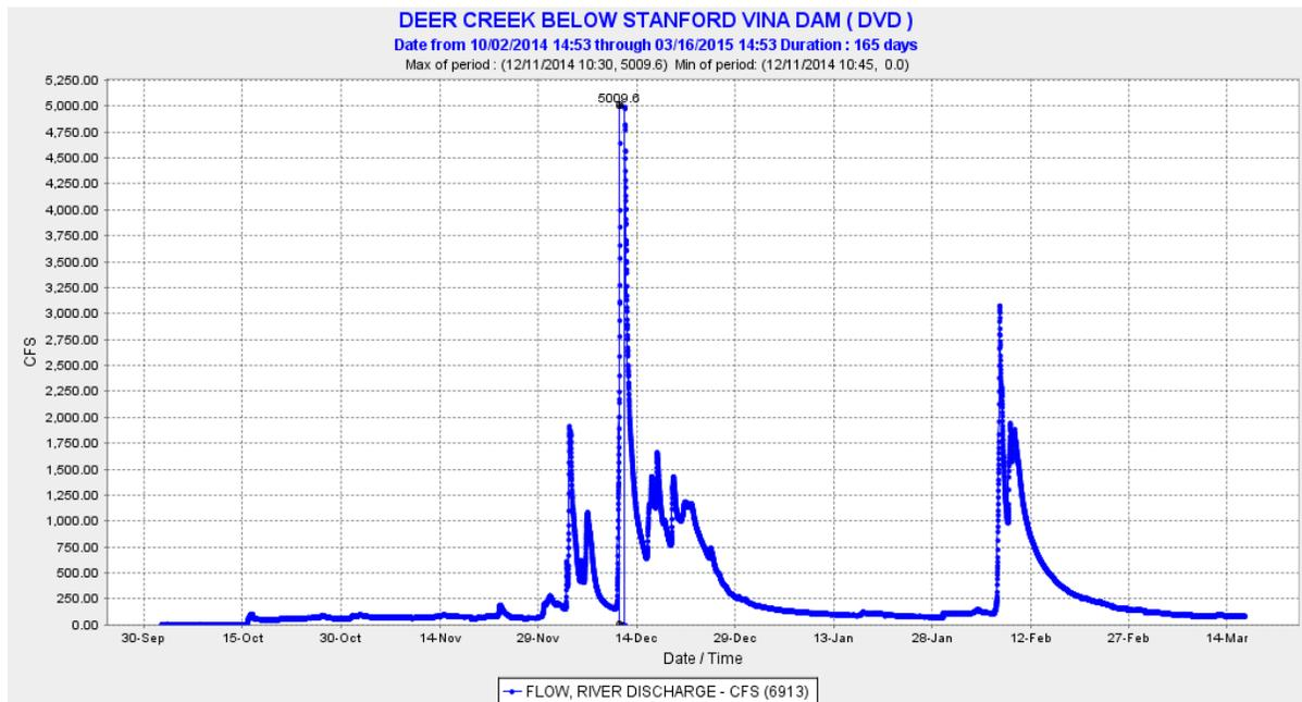
Figure 39. Deer Creek Discharge (cubic feet per second) Measured Downstream of Stanford Vina Dam (DVD) During WY2015<sup>14</sup>
