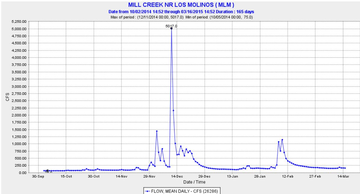
Figure 38. Mill Creek Mean Daily Flow (cubic feet per second) Measured near Los Molinos (MLM) During WY2015<sup>13</sup>
