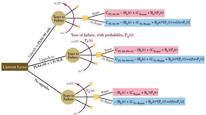
**Figure 3** Island levee decision analysis tree for assessing whether to upgrade levees and to restore islands following flooding.  $P_{ff}(t) = \text{probability of first failure at time } t$ ,  $P_f = \text{current probability of failure}$ , r = discount rate,  $B_k = \text{one year of island profits}$ .
